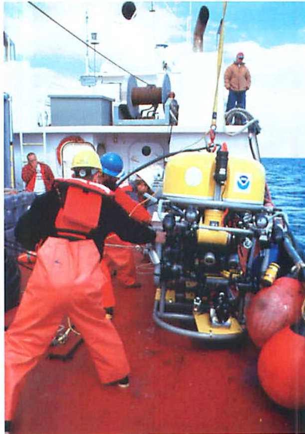
Kraken, a remotely-operated vehicle, is launched by scientists from the National Undersea Research Center (NURC), University of Connecticut. An operator at the surface directs the "robot" to specific targets for photography or sampling activities. Photo courtesy of NURC.
