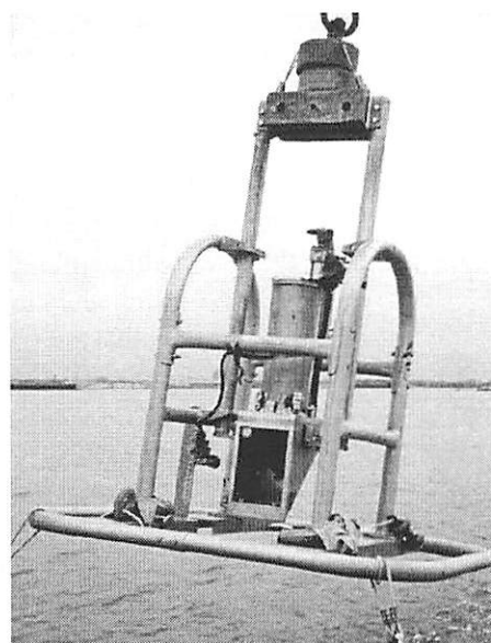
Figure 6. The sediment profile imaging (SPI) camera.
