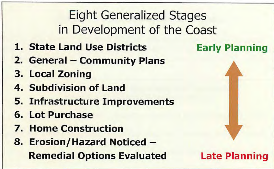
Figure 2-2 – Stages of Development and Hazard Mitigation Planning - Agencies should consider coastal erosion and other natural hazards in a process that starts at Stage 1 and continues for all subsequent development stages. It is too late in the planning process to address coastal hazards at Stage 8. This will result in severe problems and limited options for the agencies, homeowner and the public.
