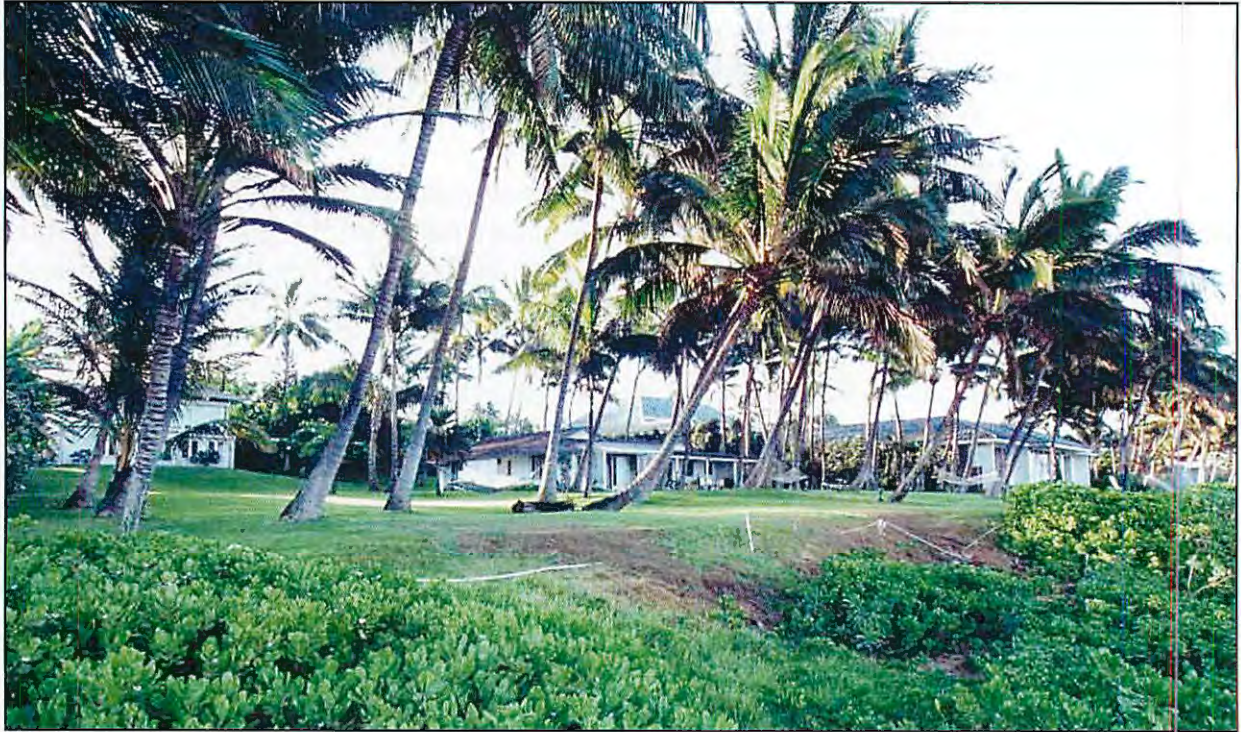
Figure 11-2 – Keawakapu Beach, Maui – Three houses with different shoreline setbacks. The house on the right is about 50 feet from the shoreline, the middle house is between 50 to 100 feet away and the house on the left, over 100 feet from the shoreline. The house on the right has a large frontyard but small backyard. The house on the left has a small frontyard and a large backyard. Because the house is farther from the shoreline and on higher ground, it is less susceptible to erosion, wave inundation and flooding.
