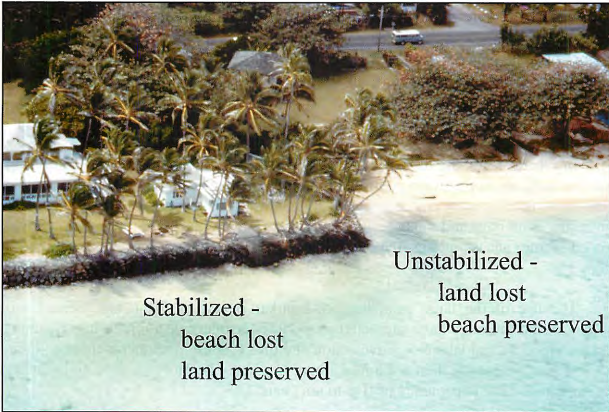
Figure 12-2 – North Shore, Oahu – For beach systems undergoing long-term retreat, stabilization with hardened structures will lead to the loss of the beach. For unstabilized shorelines, the beach is likely to remain, but migrate inland. From Fletcher, SOEST, UH.
