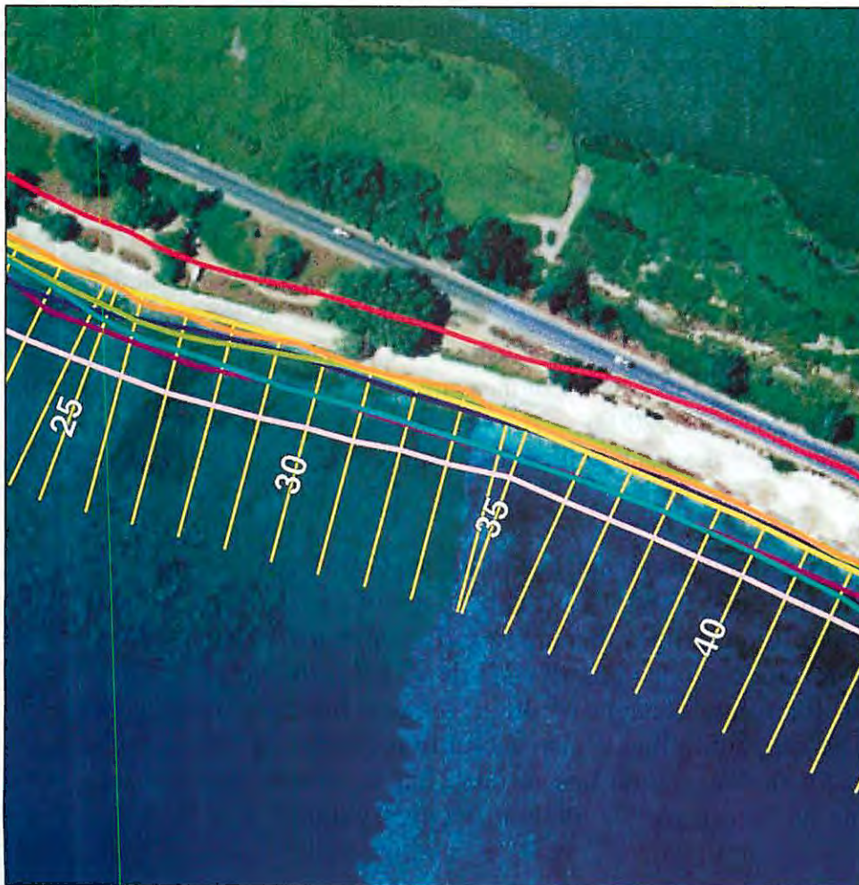
Figure 4-2 – Erosion Map of Kihei, Maui – The yellow lines perpendicular to the coast are transects from which shoreline change data are measured. The violet line along the coast is from a NOAA T sheet. The other colored lines represent positions of the beach toe on aerial photographs of different years. As the beach changes through time, erosion rates can be determined. The red line is a projection of the erosion rate times a planning period of 30 years. From the Study of Maui County, Fletcher, et al., 2002.
