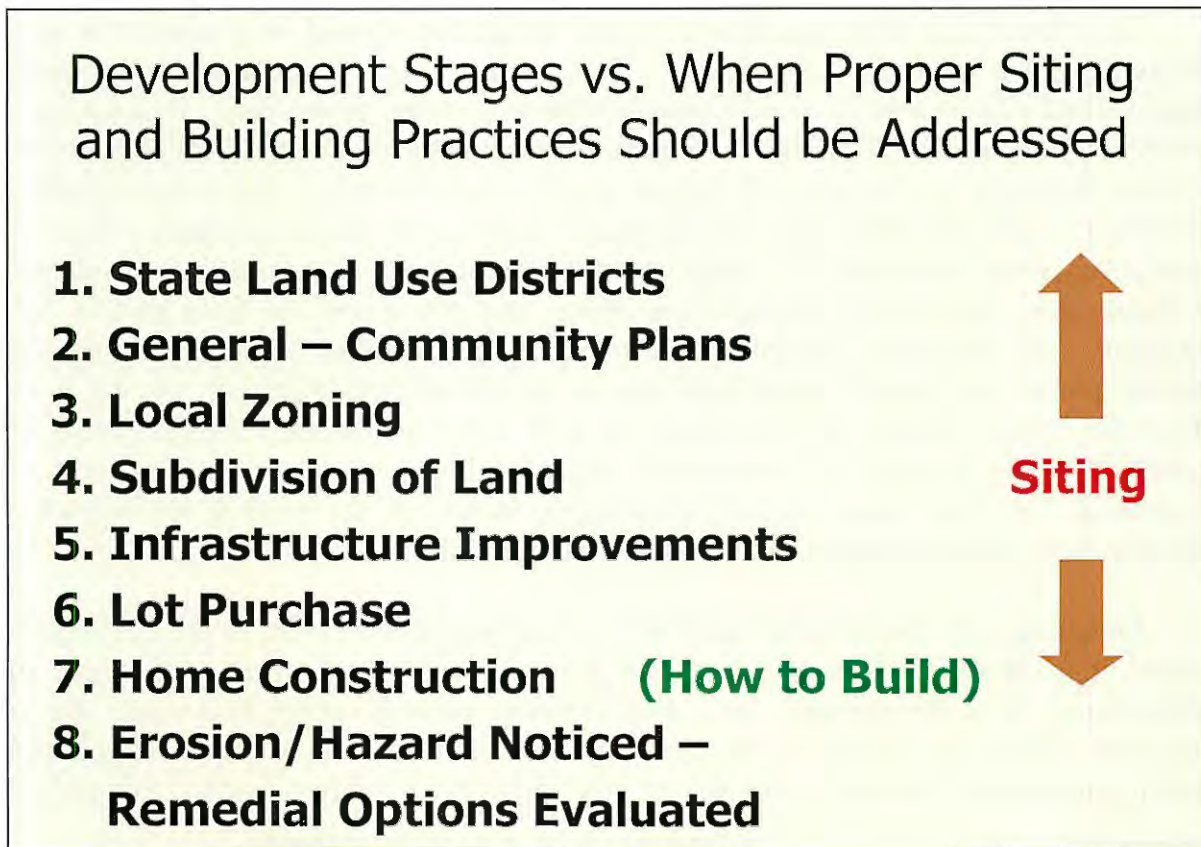
Figure 2-6 – Development Stages Versus When Siting and Building Issues are Addressed - Siting correctly and building correctly are the two keys to the proper mitigation of coastal hazards. For legal, political and practical purposes, siting issues should be addressed as early as possible in the development process (stages 1 through 4). Siting at stages 5 through 8 may be done correctly, but is likely to be improper due to prior development decisions that become irreversible. Building correctly can be done at Stage 7. See footnote 7 on definition of siting.
