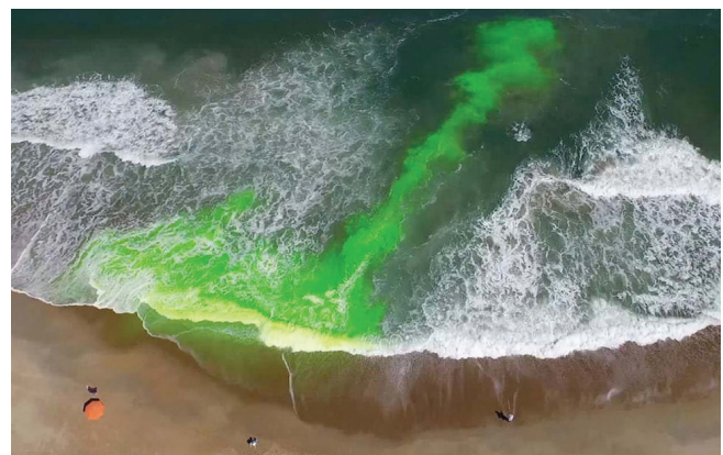
A photo of a rip current highlighted by harmless green dye. Photo credit: NOAA
