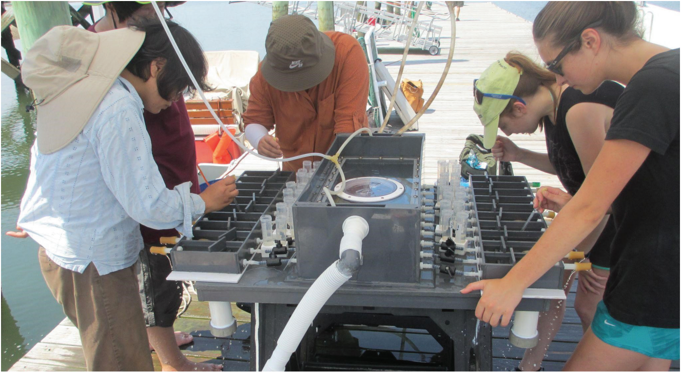
Field experiments to measure feeding and nutrient uptake by shellfish in the Greenwich watershed in 2015. Photo credit: NOAA Fisheries
