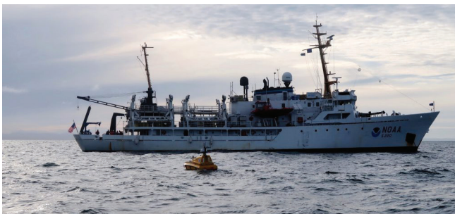
The University of New Hampshire's Bathymetric Explorer and Navigator (BEN) uncrewed surface vehicle launched from NOAA Ship Fairweather . Photo credit: Christina Belton, NOAA
