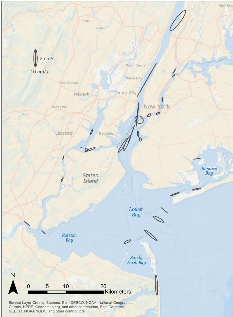
Figure 6-5. K_1 tidal ellipses for the entire study region. Note that these are on a different scale than M_2 in order to see the ellipses. These data are at about 1/8 the scale of the M_2 data.
