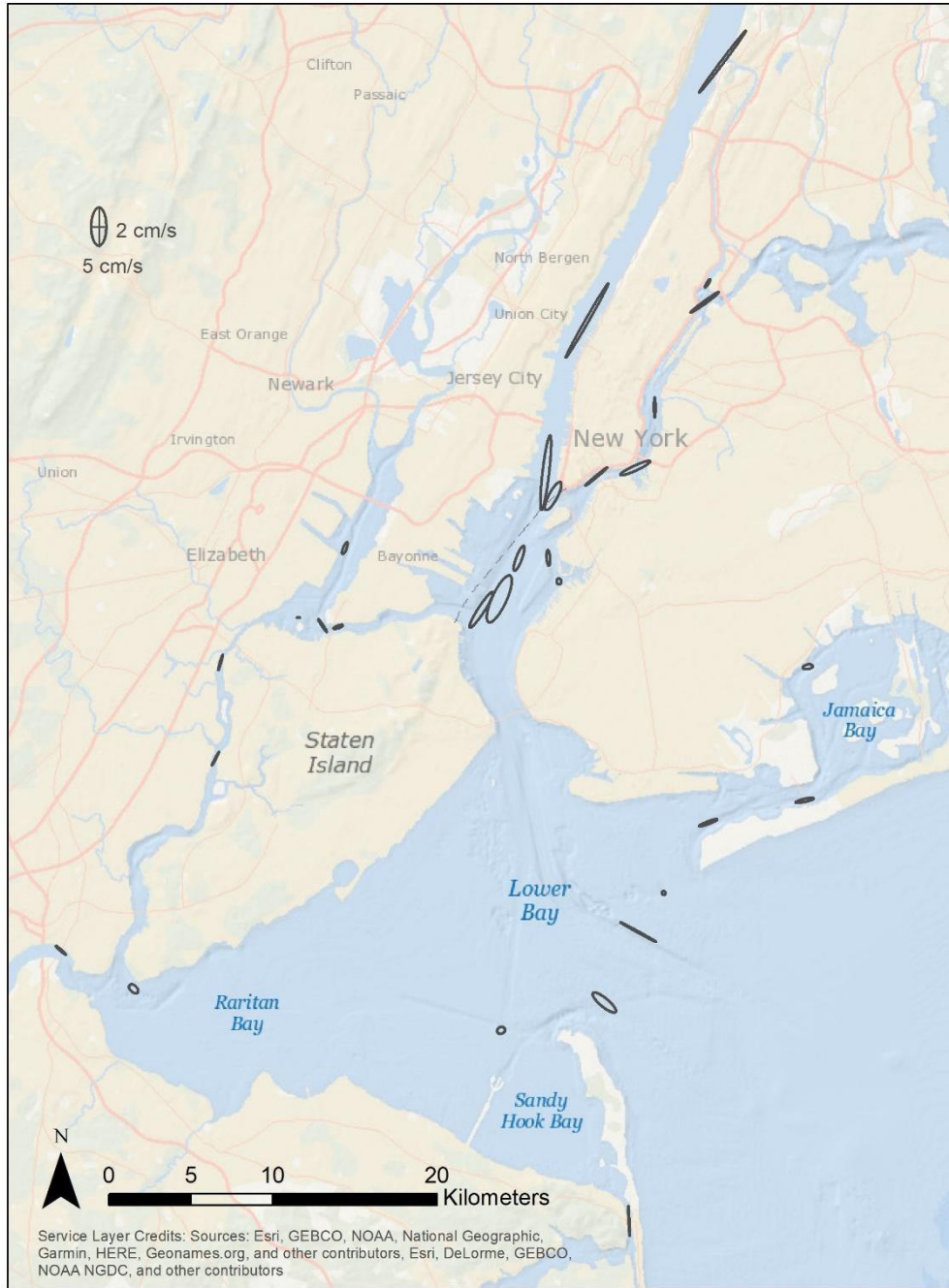
Figure 6-4. O_1 tidal ellipses for the entire study region. Note that these are on a different scale than M_2 in order to see the ellipses. These data are at about 1/15 the scale of the M_2 data.
