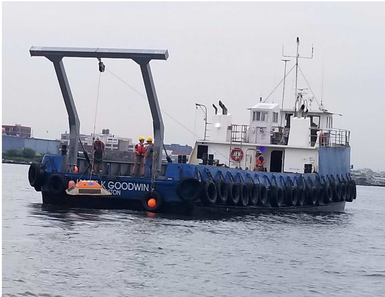
Figure 3-1. R/V James K Goodwin deploying a trawl-resistant bottom mount (TRBM) in the East River.
