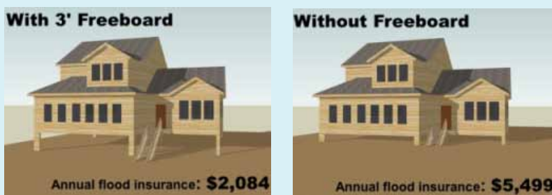
Figure 2-6. In this example, adding a small amount of height has very little effect on the look of a home, but resulted in a substantial flood insurance savings. 8
