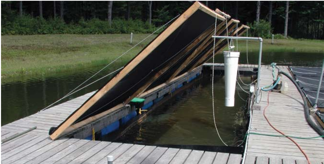
7.7 Floating raceway with screening lids and automatic feeders. Chris Hartleb
