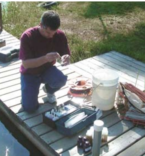
2.5 Using a HACH kit to measure ammonia or nitrite. Chris Hartleb
