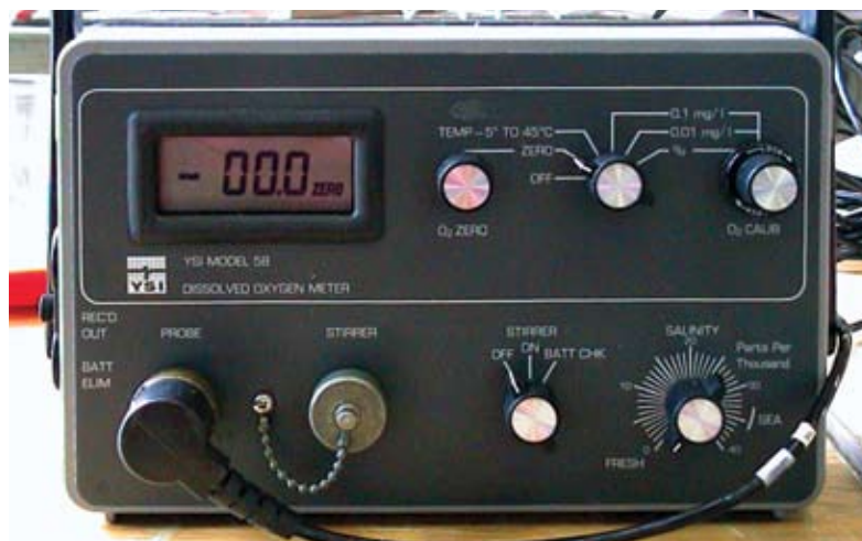
2.3 A DO meter checks temperature and dissolved oxygen. James A. Held
