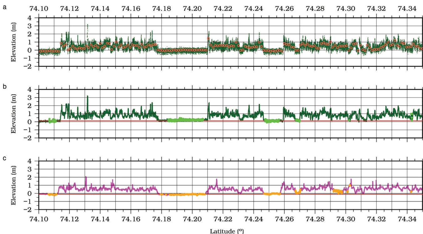
Fig. 4. Sea-ice elevation measured along-track in case-study region 4. (a) MABEL elevations from beam 6, after application of surface-finding algorithm. (b) Same as for (a), after application of 10 m along-track filter. (c) ATM elevation profile. Lighter-color dots (light-green (b) and orange (c)) indicate the location, and height, of lead elevation measurements, after application of lead discrimination threshold derived from DMS imagery (Fig. 2e). Red line (b, c) indicates sea surface height, interpolated along-track. Open red circles (a) indicate a set of simulated surface elevations assuming the ICESat sampling configuration. Segment shown is \sim 28 km long.
