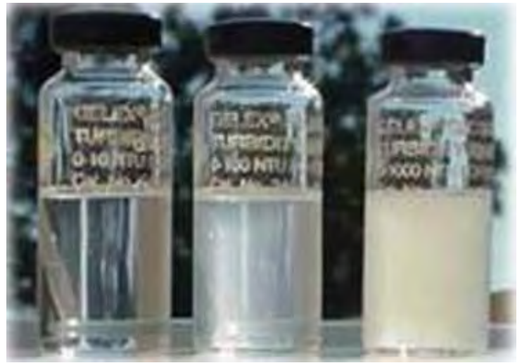
Figure 2-6. From left to right, turbidity standards 5, 50, and 500 Nephelometric Turbidity Units or NTUs. The higher the NTU value, the more turbid the standard. Notice how the far right sample is white (more turbid) than the far left standard (almost clear). Referenced from the U.S. Geological Survey.
