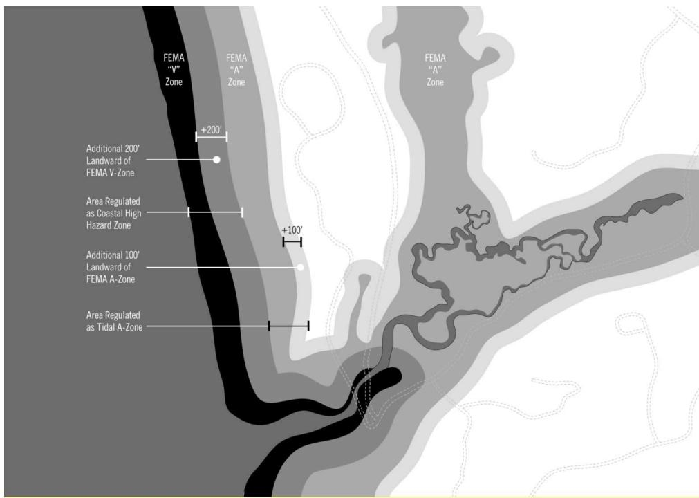
Diagram: The above diagram illustrates the delineation of the Coastal High Hazard Zone and the Tidal A-Zone as defined above in Article 3 (1) and (2). These zones together comprise the Coastal Floodplain District regulated by this bylaw.
