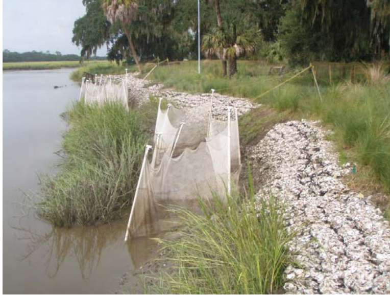
Figure 9. Picture of bottomless lift nets deployed at low tide, prior to sampling, over a living shoreline on Little St. Simons Island, GA.
