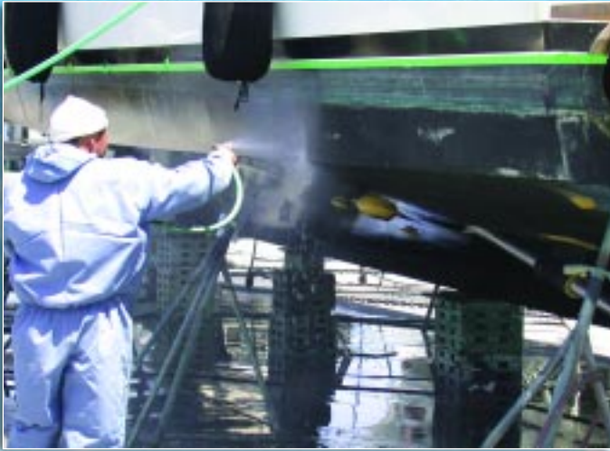
Hydro-Washing at Boat Repair Yard
