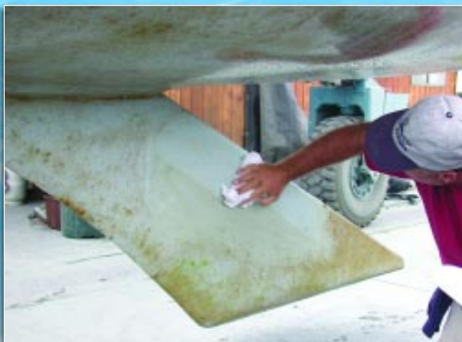
Sailboat-Ceramic Epoxy (5 months): Cleaning with Soft Rag
