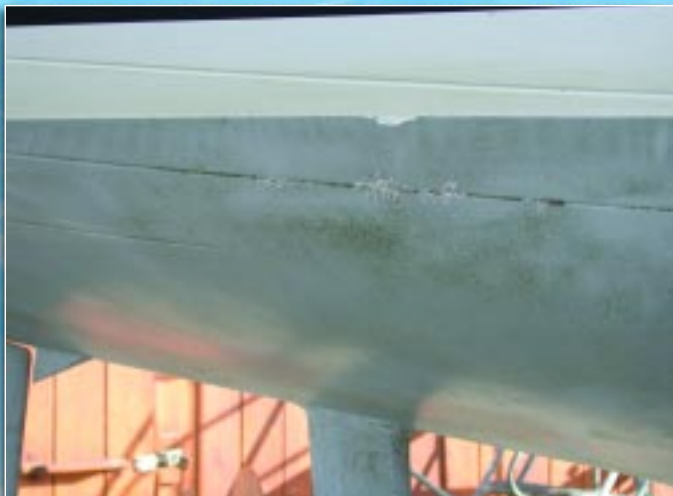
Powerboat-Ceramic-Epoxy (14 months): With Tubeworm Remnants
