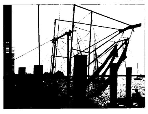
a Vietnamese "chopstick" rig, is pushed in pairs — one net on each side of the boat — rather than towed behind like an otter trawl.
