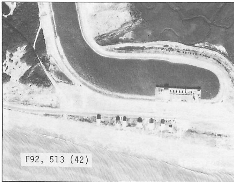
Figure 92. Coolant water from the atomic energy electrical generating facility near Southport is carried in this canal. It crosses the Intracoastal Waterway and reaches the sea in the vicinity of Yaupon Beach.
