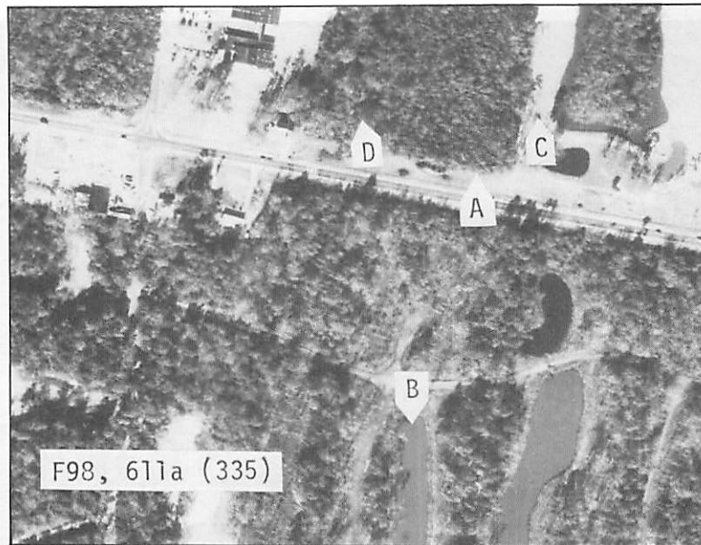
Figure 98. Point A indicates a low, wet place between the dunes at C and D. The appearance of the mixed deciduous and coniferous vegetation indicated by A is different in texture from the maritime forest vegetation on both sides of the road from D. The trough in which A is located continues across the road to point B where it is very low and filled with fresh water and should be classified as 521.
