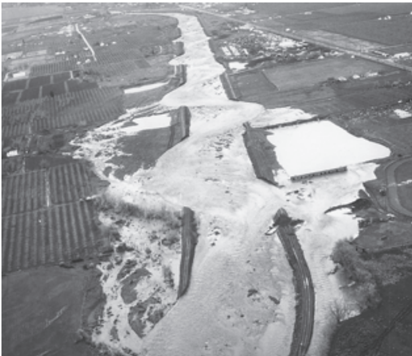
Figure 11. Walla Walla River (1964 flood showing meanders in a channelized section near Milton-Freewater). (OSU Archives)
