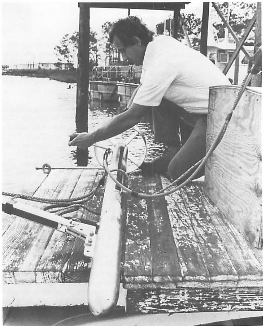
NORDA geologist Peter Fleischer checks torpedo-like towfish used in sonic survey for misplaced bridge rubble in Alabama waters.
