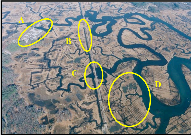
Figure 2.2. Human impacts such as: A.) filling of marsh for development, B.) installation of railroad on the marsh surface, C.) tidal restriction, and D.) grid ditches affect the Hampton-Seabrook estuary.
