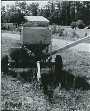
Tractor-powered blower for feeding fish in ponds
