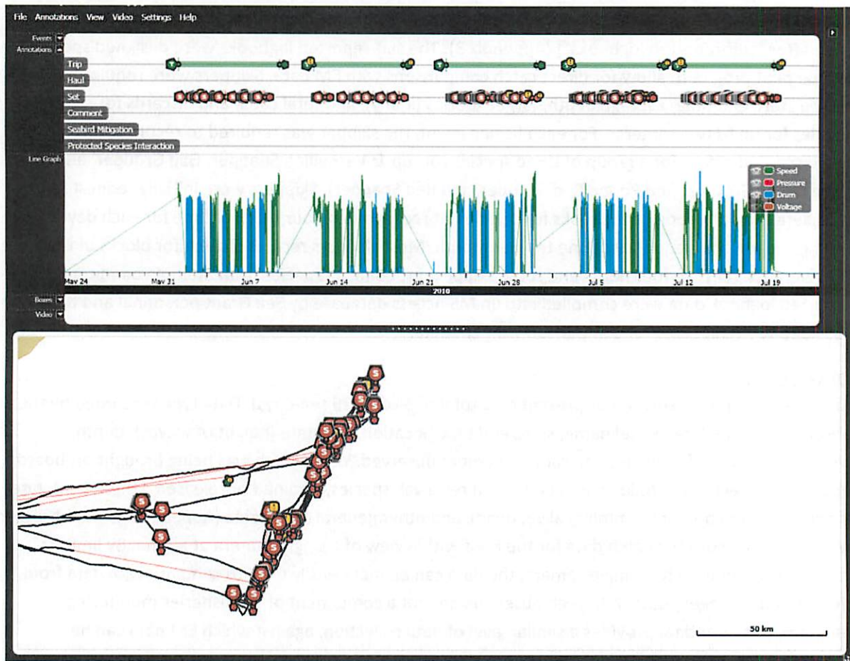
Figure 4. Example of a complete data set as seen in EM Interpret with annotations for trips and fishing events (sets).
