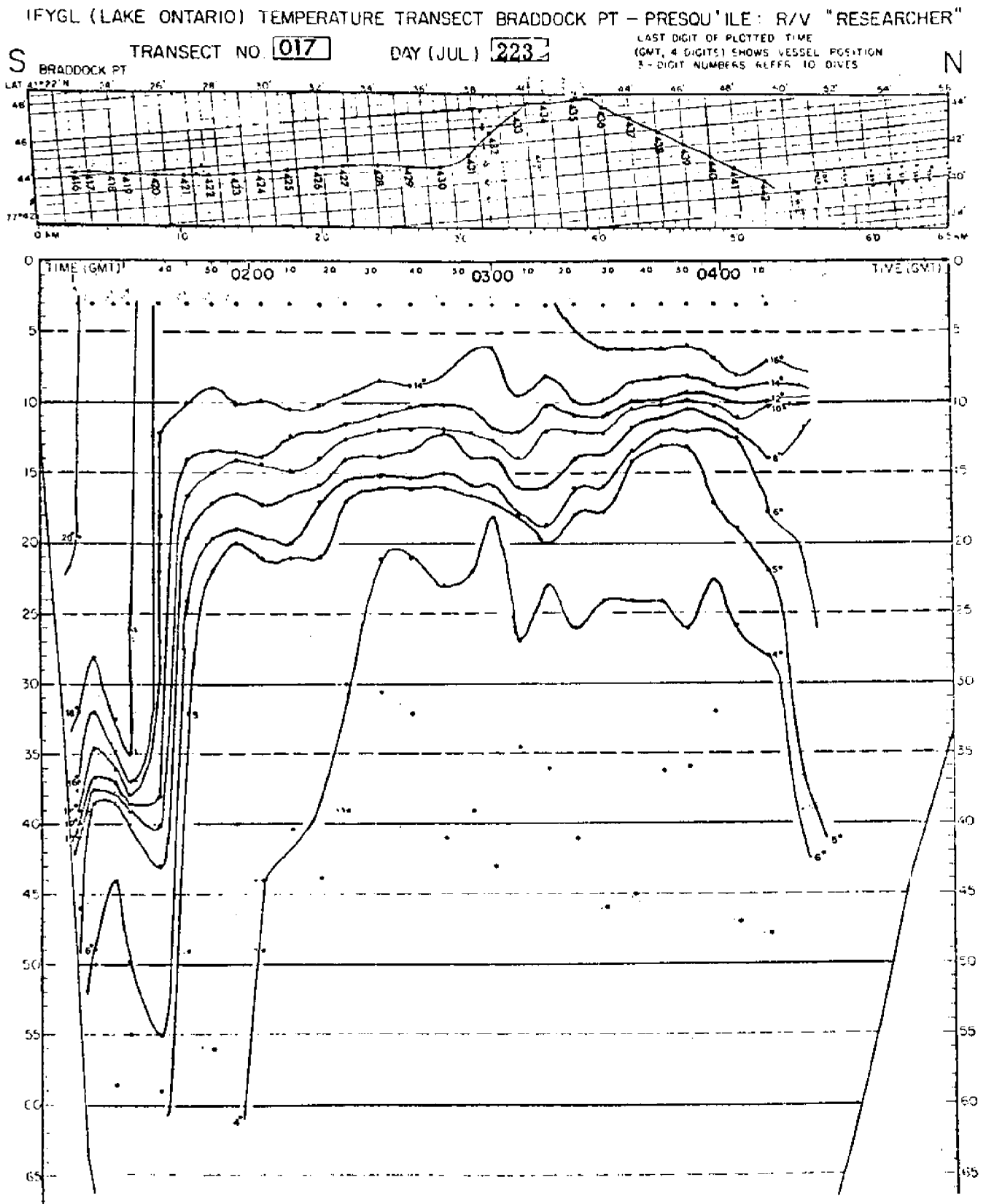
Figure 19 Temperature distribution across transect of Lake Ontario from Braddock Point to Presqu'ile for 10 August 1972, 0100-0400 GMT.
