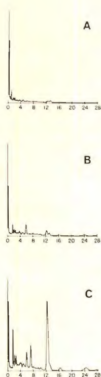
Fig. 2. Electron capture gas chromatographic traces of hexane extracts of tidepool water. The water samples were obtained from an isolated tidepool at low tide and extracted immediately. At the time of sampling, the air temperature was 27°C, the water temperature was 18.5°C and the day was partly cloudy. Neither Nanograde hexane nor 1 liter of Nanograde hexane condensed to 5ml contained any contaminating material. A) Time zero, 4 \mu l; B) 1.5 hours, 4 \mu l; C) 3 hours, 4 \mu l
