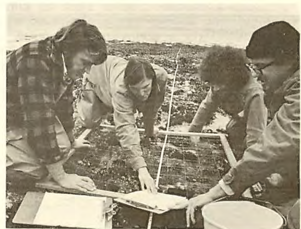
Dr. John Pearse (left) and student team enumerating the intertidal transect near Natural bridges State Park, Santa Cruz County. The wood square represents a meter quadrat which has been subdivided into ten 10cm squares.
