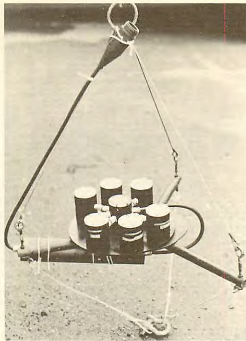
Sea floor light unit with six spectral region sensors shown during early trials before its installation on the sea floor.
