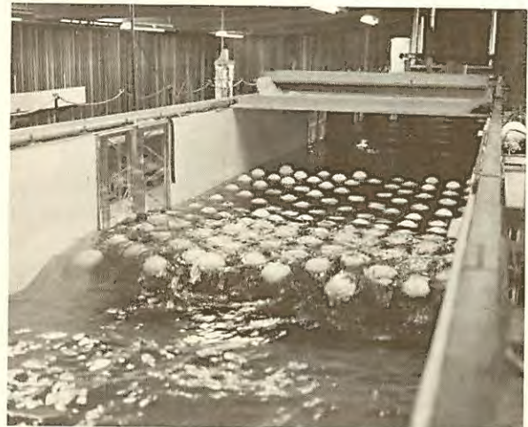
Tethered float breakwater experiment in laboratory wave channel showing attenuation of simulated ocean waves coming from lower left.
