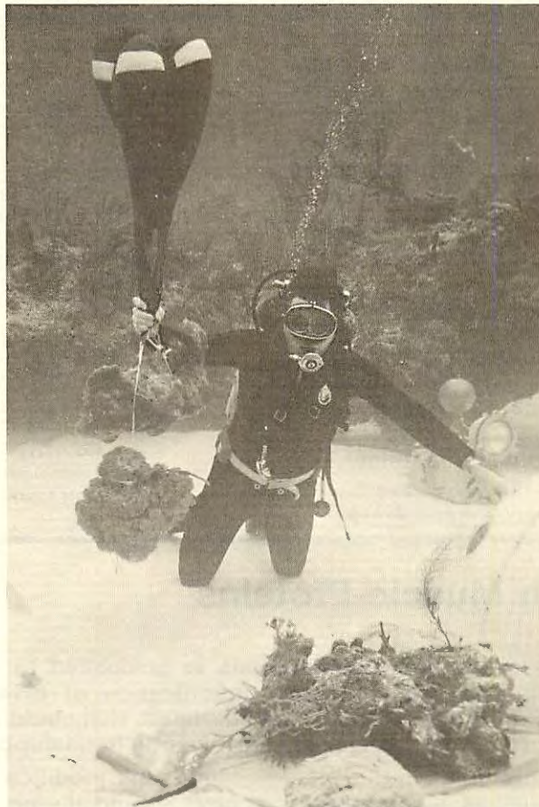
Dr. L. H. DiSalvo carries reef subsamples (coral heads) to respirometer dome (right) to measure oxygen consumption rates.
