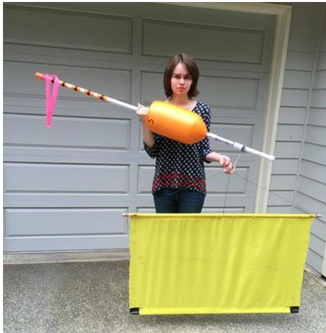
Figure 4. Windowshade drogue and marker float as described in the text.
