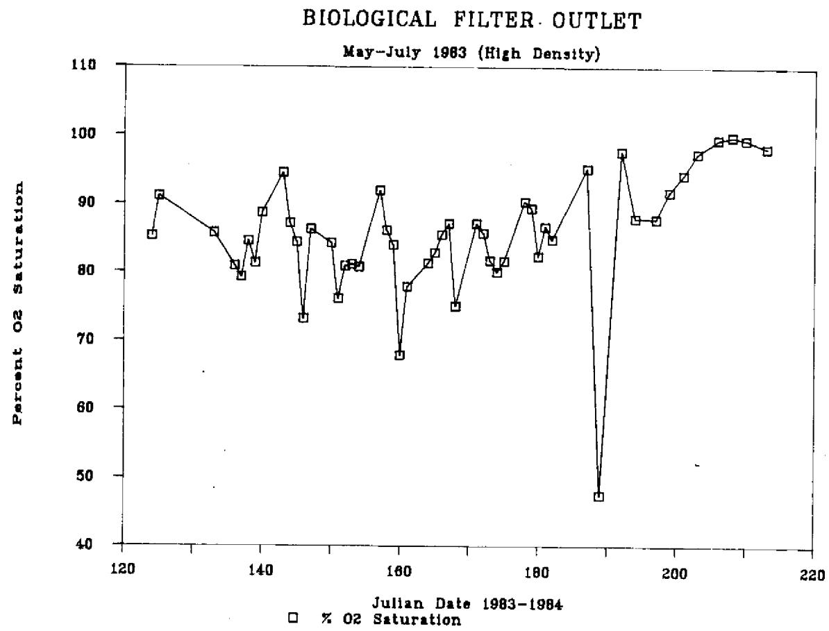
Figure 6. Mean outlet oxygen-saturation levels for the biological filter stocked at high densities (May-July, 1983)
