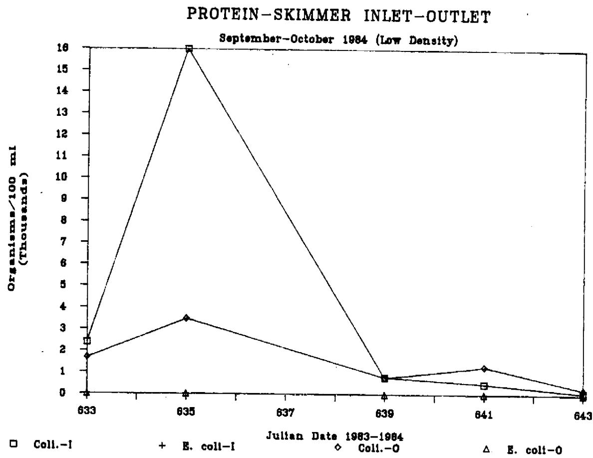
Figure 30. MPN total coliform and MPN E. coli inlet and outlet populations for the protein skimmer stocked at low densities (September-October, 1984)
