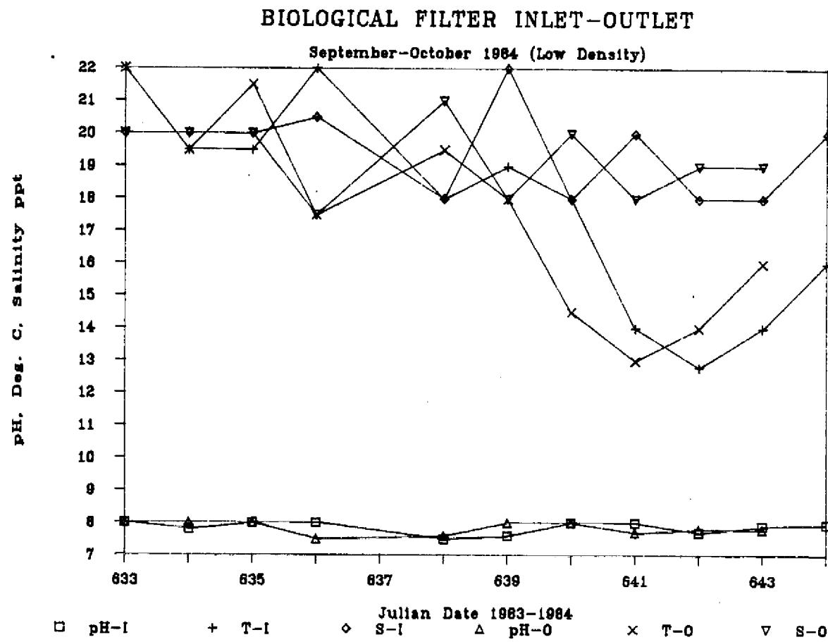
Figure 2. Inlet and outlet pH, temperature ( $^{\circ}\text{C}$ ), and salinity (ppt) levels for the biological filter stocked at low densities (September-October, 1984)
