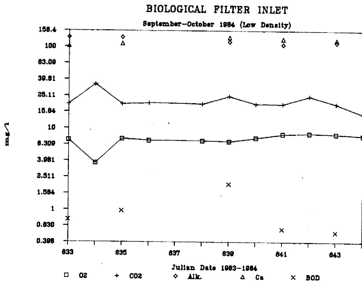
Figure 4. Mean inlet dissolved O<sub>2</sub>, dissolved CO<sub>2</sub>, alkalinity, calcium, and BOD levels for the biological filter stocked at low densities (September-October, 1984)
