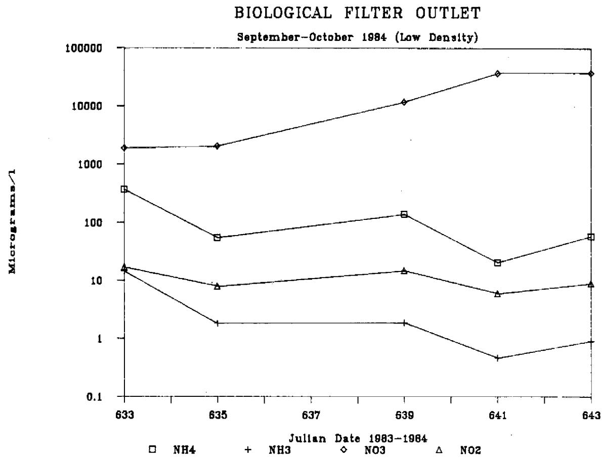
Figure 10. Mean outlet ammonium ( $\text{NH}_4$ ), ammonia ( $\text{NH}_3$ ), nitrate ( $\text{NO}_3$ ), and nitrite ( $\text{NO}_2$ ) levels for the biological filter stocked at low densities (September-October, 1984)
