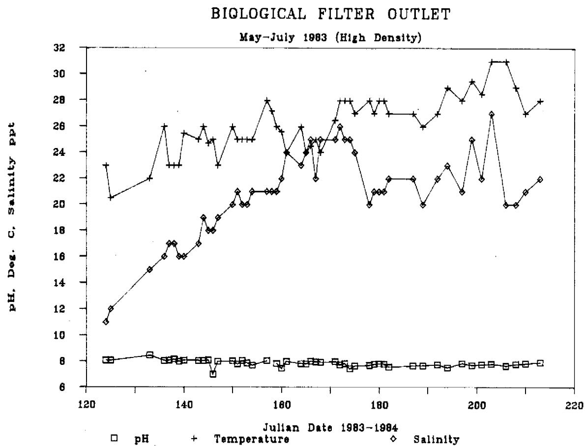
Figure 1. Outlet pH, temperature ( $^{\circ}\text{C}$ ), and salinity (ppt) levels for the biological filter stocked at high densities (May-July, 1983)
