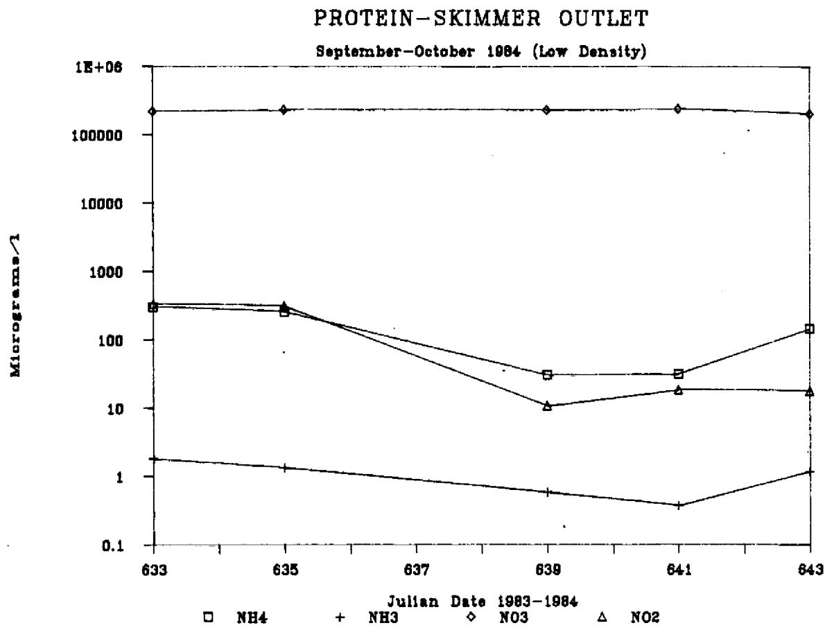
Figure 26. Mean outlet ammonium ( $\text{NH}_4$ ), ammonia ( $\text{NH}_3$ ), nitrate ( $\text{NO}_3$ ), and nitrite ( $\text{NO}_2$ ) levels for the protein skimmer stocked at low densities (September-October, 1984)
