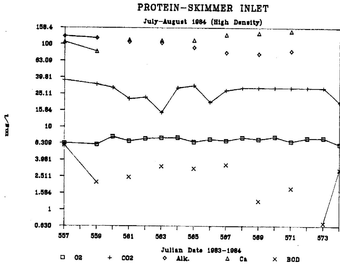
Figure 17. Mean inlet dissolved O<sub>2</sub>, dissolved CO<sub>2</sub>, alkalinity, calcium, and BOD levels for the protein skimmer stocked at high densities (July-August, 1984)
