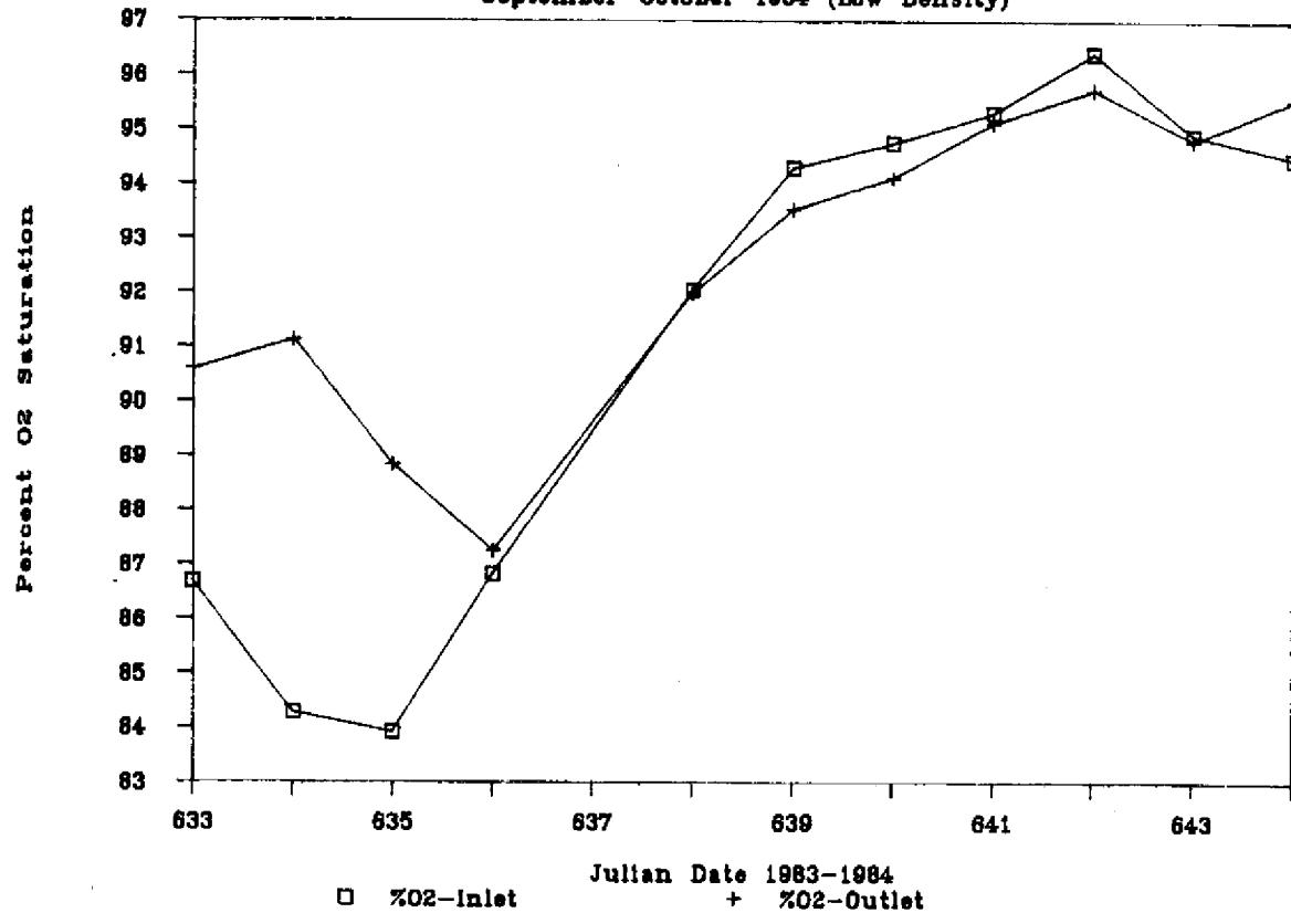
Figure 22. Mean inlet and outlet oxygen-saturation levels for the protein skimmer stocked at low densities (September-October, 1984)
