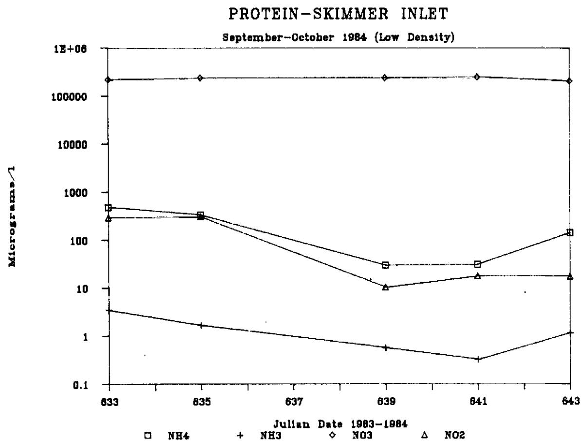
Figure 25. Mean inlet ammonium ( $\text{NH}_4$ ), ammonia ( $\text{NH}_3$ ), nitrate ( $\text{NO}_3$ ), and nitrite ( $\text{NO}_2$ ) levels for the protein skimmer stocked at low densities (September-October, 1984)
