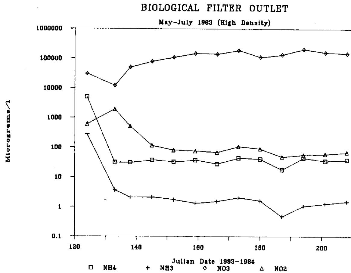
Figure 8. Mean outlet ammonium ( $\text{NH}_4$ ), ammonia ( $\text{NH}_3$ ), nitrate ( $\text{NO}_3$ ), and nitrite ( $\text{NO}_2$ ) levels for the biological filter stocked at high densities (May-July, 1983)
