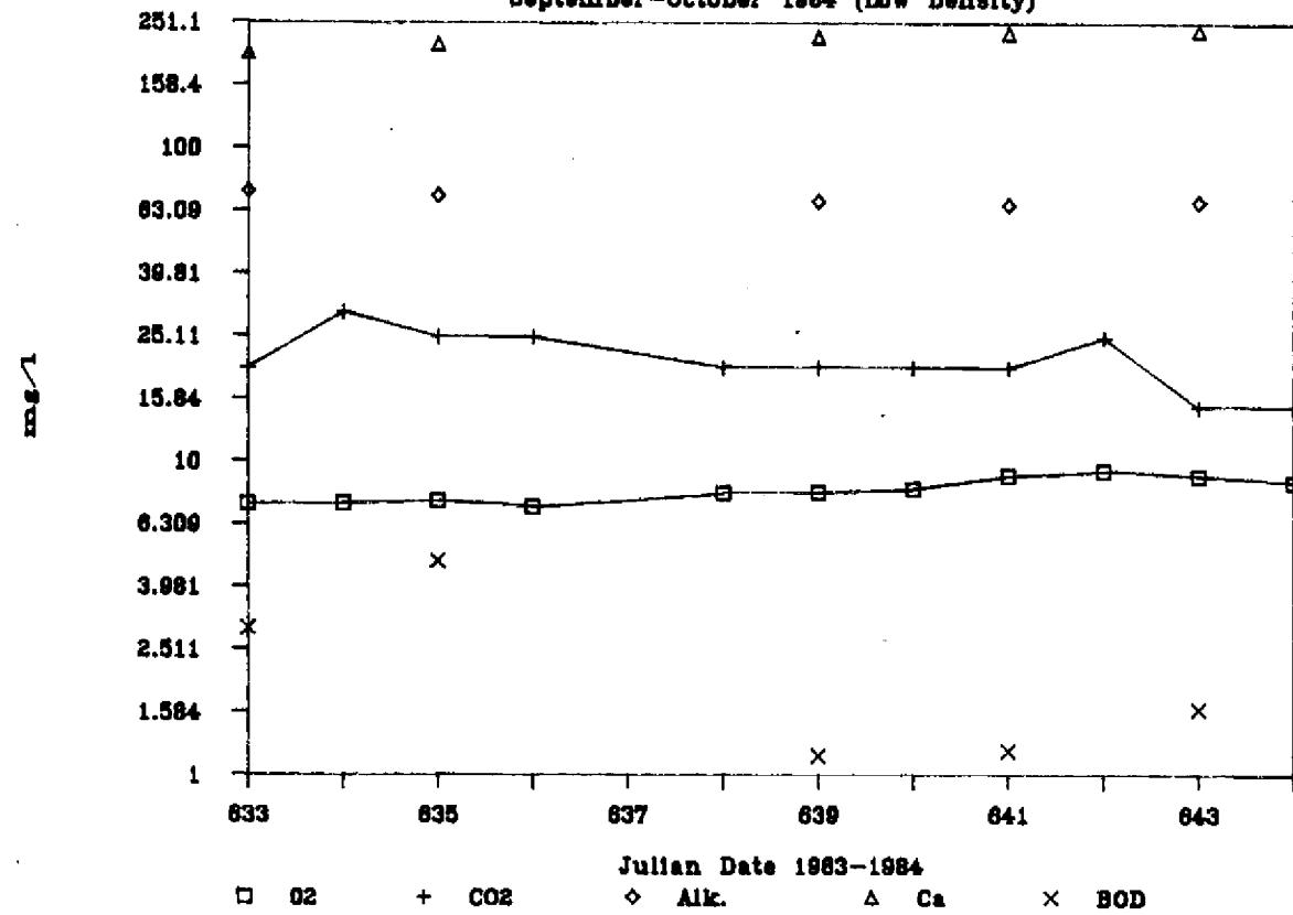
Figure 20. Mean outlet dissolved  $\text{O}_2$ , dissolved  $\text{CO}_2$ , alkalinity, calcium, and BOD levels for the protein skimmer stocked at low densities (September-October, 1984)
