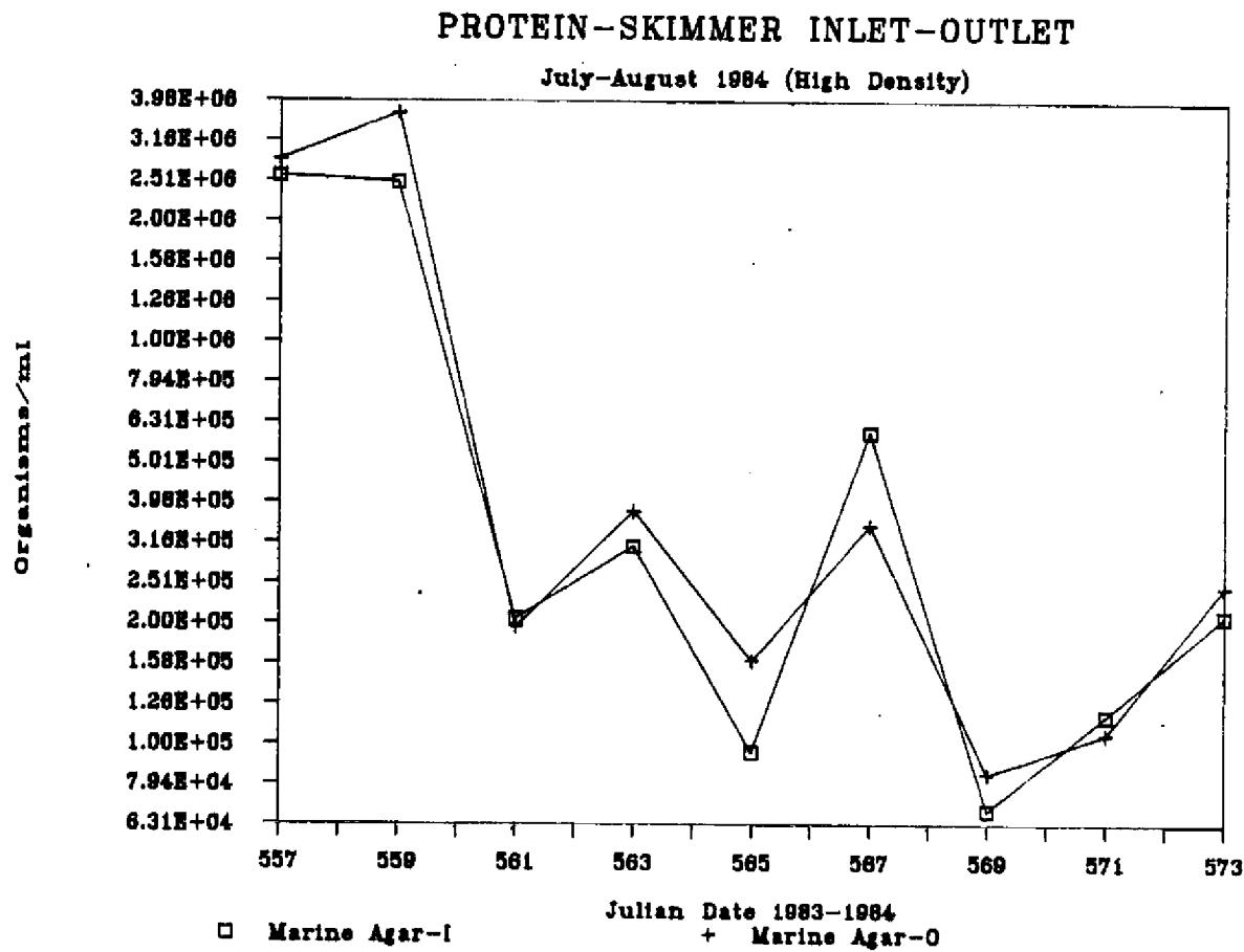
Figure 27. Mean inlet and outlet marine agar plate counts for the protein skimmer stocked at high densities (July-August, 1984)
