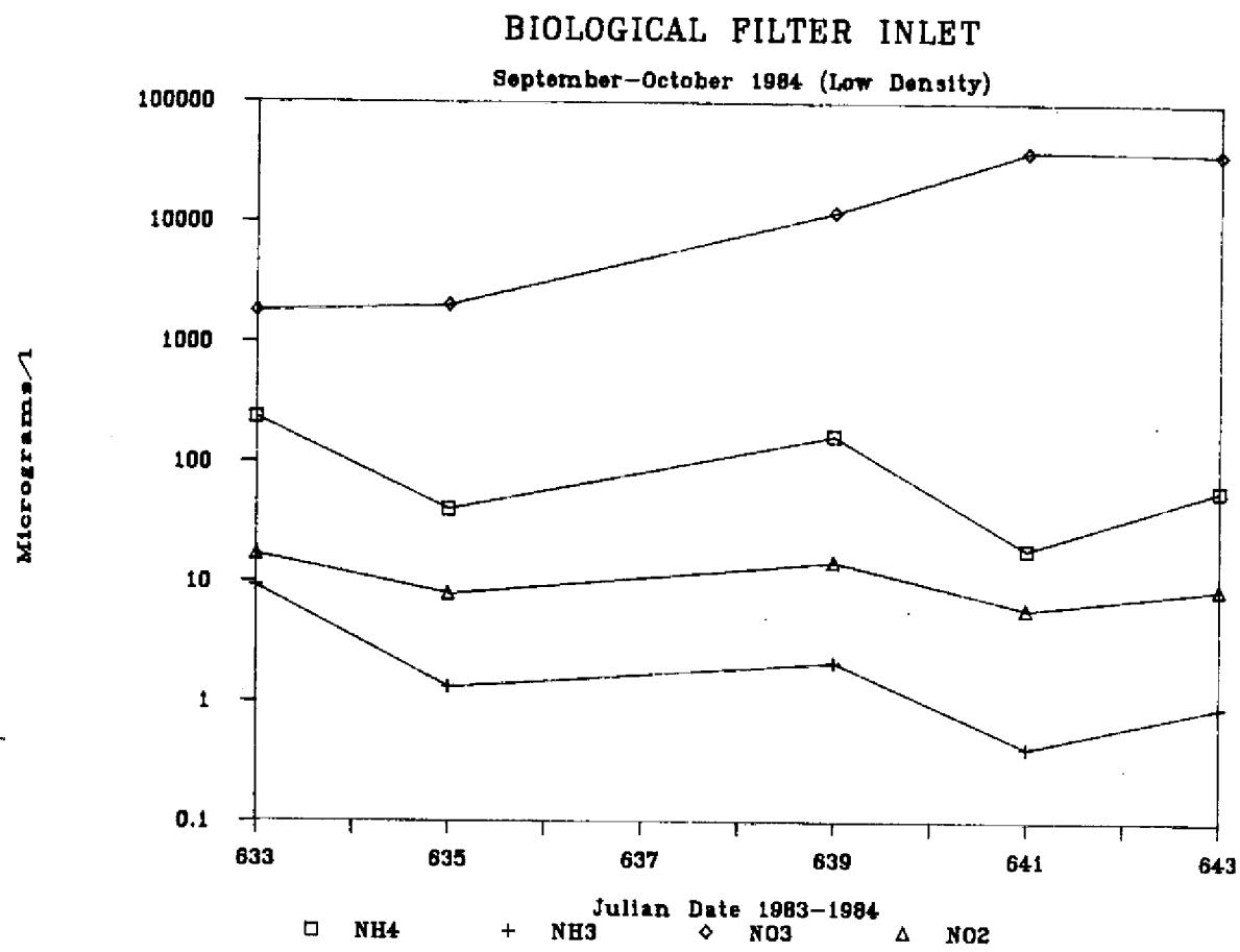
Figure 9. Mean inlet ammonium ( $\text{NH}_4$ ), ammonia ( $\text{NH}_3$ ), nitrate ( $\text{NO}_3$ ), and nitrite ( $\text{NO}_2$ ) levels for the biological filter stocked at low densities (September-October, 1984)
