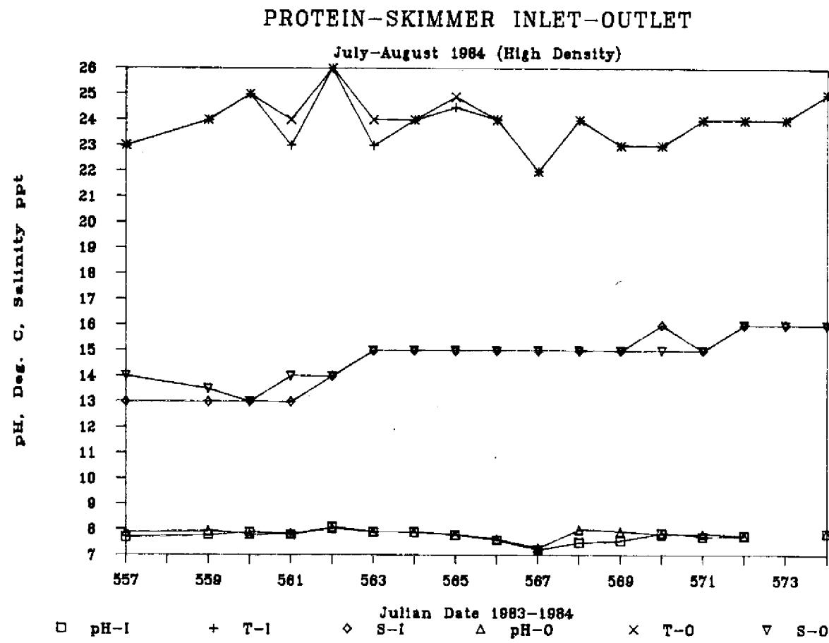
Figure 15. Inlet and outlet pH, temperature ( $^{\circ}\text{C}$ ), and salinity (ppt) levels for the protein skimmer stocked at high densities (July-August, 1984)
