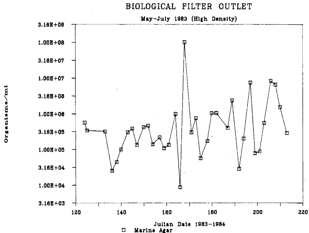
Figure 11. Mean outlet marine agar plate counts for the biological filter stocked at high densities (May-July, 1983)
