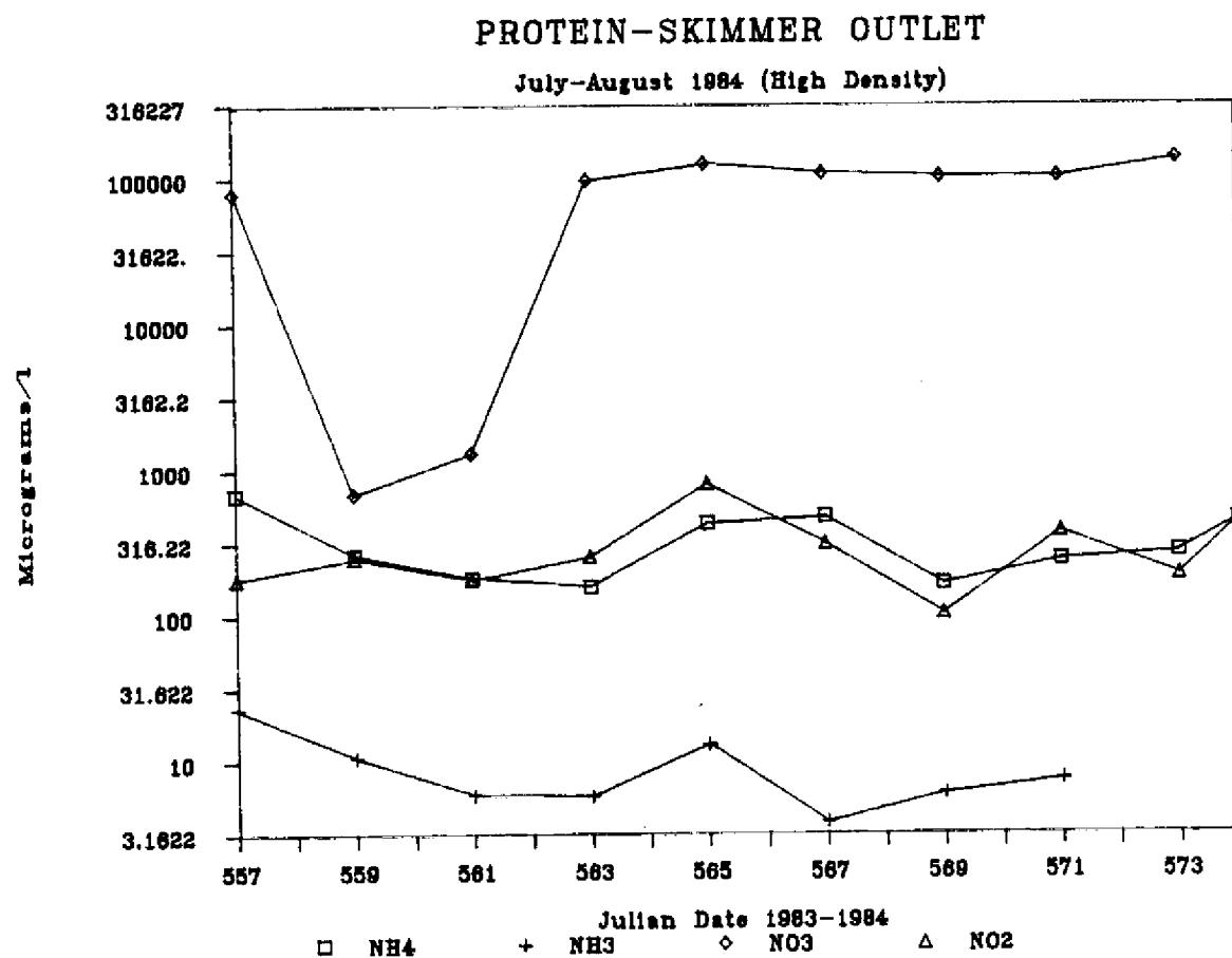
Figure 24. Mean outlet ammonium ( $\text{NH}_4$ ), ammonia ( $\text{NH}_3$ ), nitrate ( $\text{NO}_3$ ), and nitrite ( $\text{NO}_2$ ) levels for the protein skimmer stocked at high densities (July-August, 1984)
