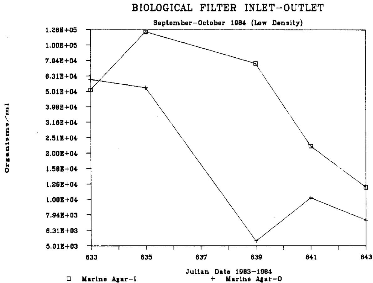
Figure 12. Mean inlet and outlet marine agar plate counts for the biological filter stocked at low densities (September-October, 1984)
