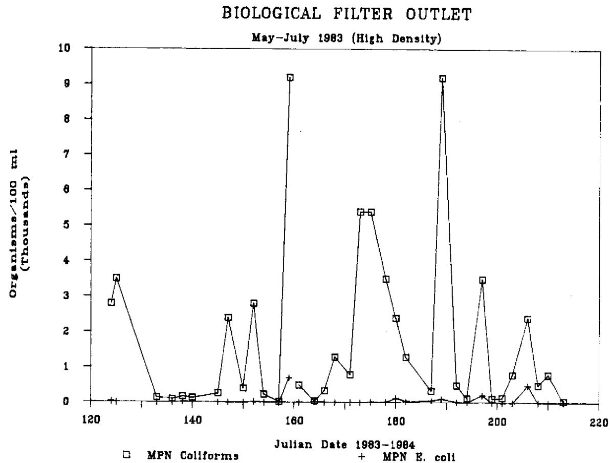
Figure 13. MPN total coliform and MPN *E. coli* outlet populations for the biological filter stocked at high densities (May-July, 1983)
