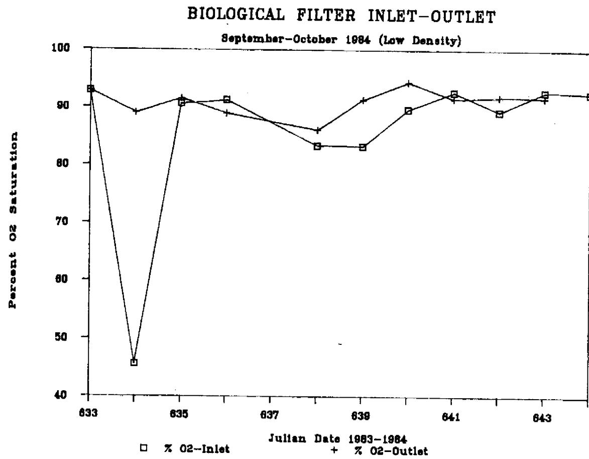
Figure 7. Mean inlet and outlet oxygen-saturation levels for the biological filter stocked at low densities (September-October, 1984)
