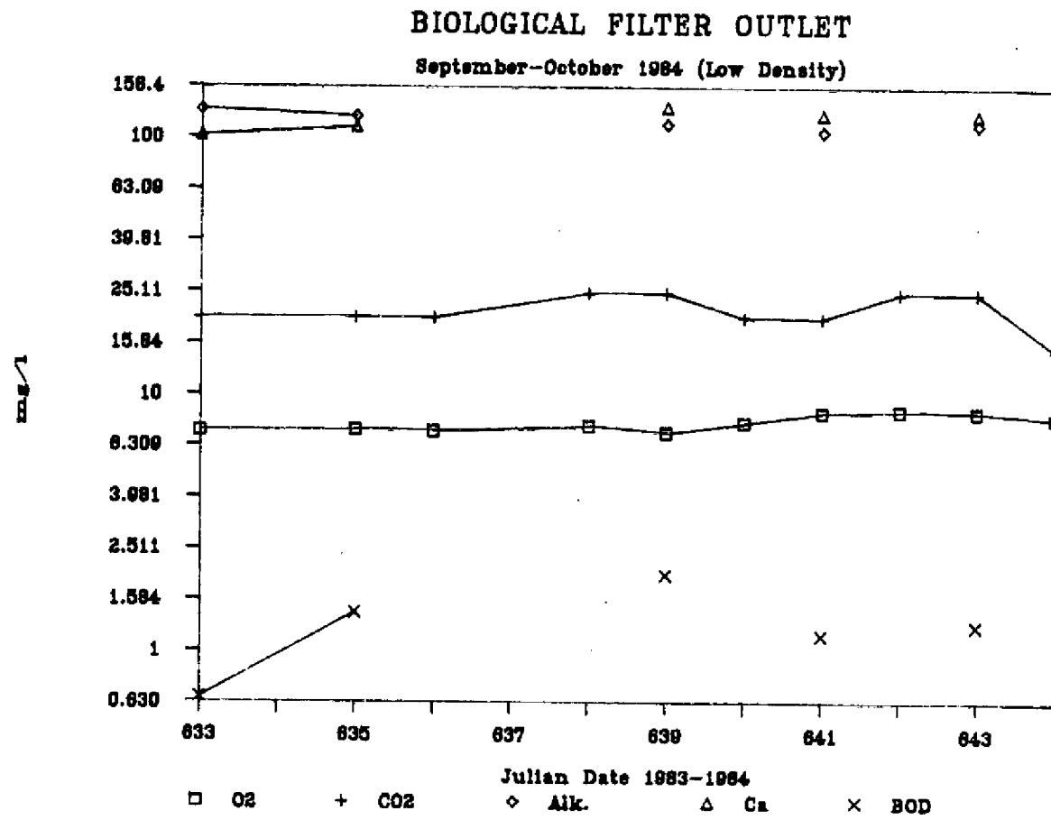
Figure 5. Mean outlet dissolved O<sub>2</sub>, dissolved CO<sub>2</sub>, alkalinity, calcium, and BOD levels for the biological filter stocked at low densities (September-October, 1984)
