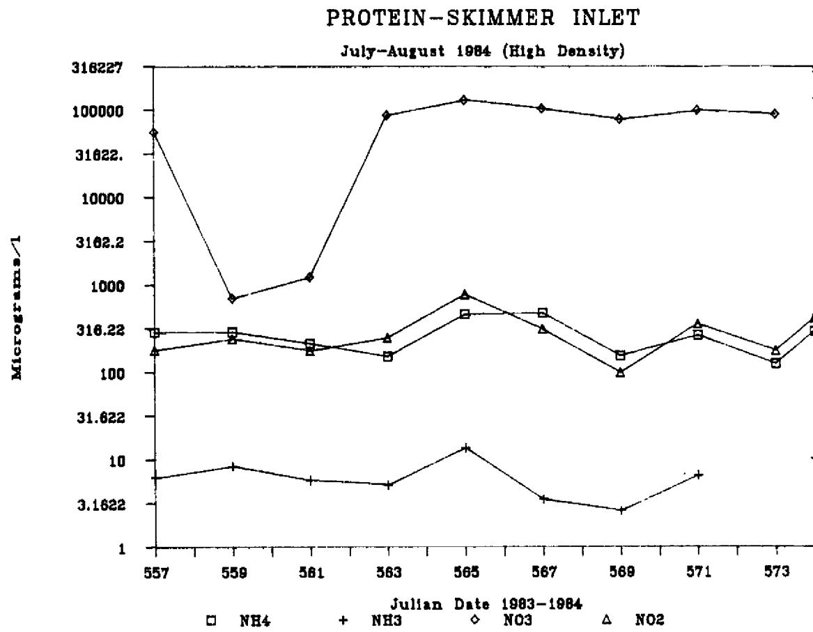
Figure 23. Mean inlet ammonium ( $\text{NH}_4$ ), ammonia ( $\text{NH}_3$ ), nitrate ( $\text{NO}_3$ ), and nitrite ( $\text{NO}_2$ ) levels for the protein skimmer stocked at high densities (July-August, 1984)
