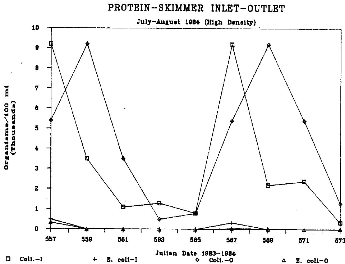
**Figure 29.** MPN total coliform and MPN E. coli inlet and outlet populations for the protein skimmer stocked at high densities (July-August, 1984)
