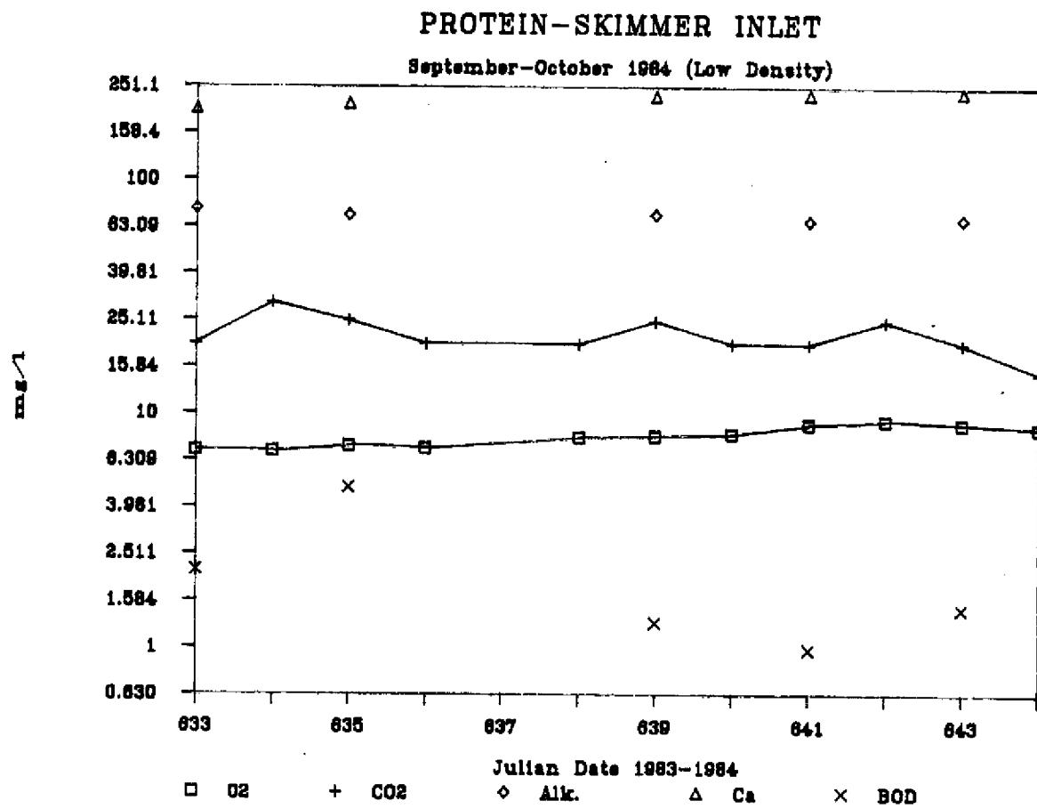
Figure 19. Mean inlet dissolved  $\text{O}_2$ , dissolved  $\text{CO}_2$ , alkalinity, calcium, and BOD levels for the protein skimmer stocked at low densities (September-October, 1984)
