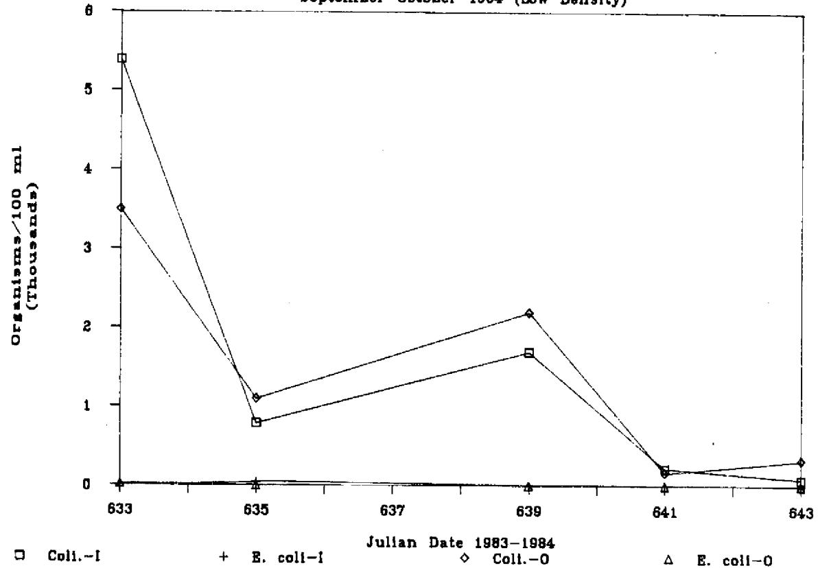
Figure 14. MPN total coliform and MPN *E. coli* inlet and outlet populations for the biological filter stocked at low densities (September-October, 1984)
