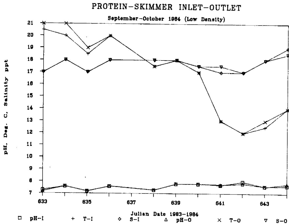
Figure 16. Inlet and outlet pH, temperature ( $^{\circ}\text{C}$ ), and salinity (ppt) levels for the protein skimmer stocked at low densities (September-October, 1984)
