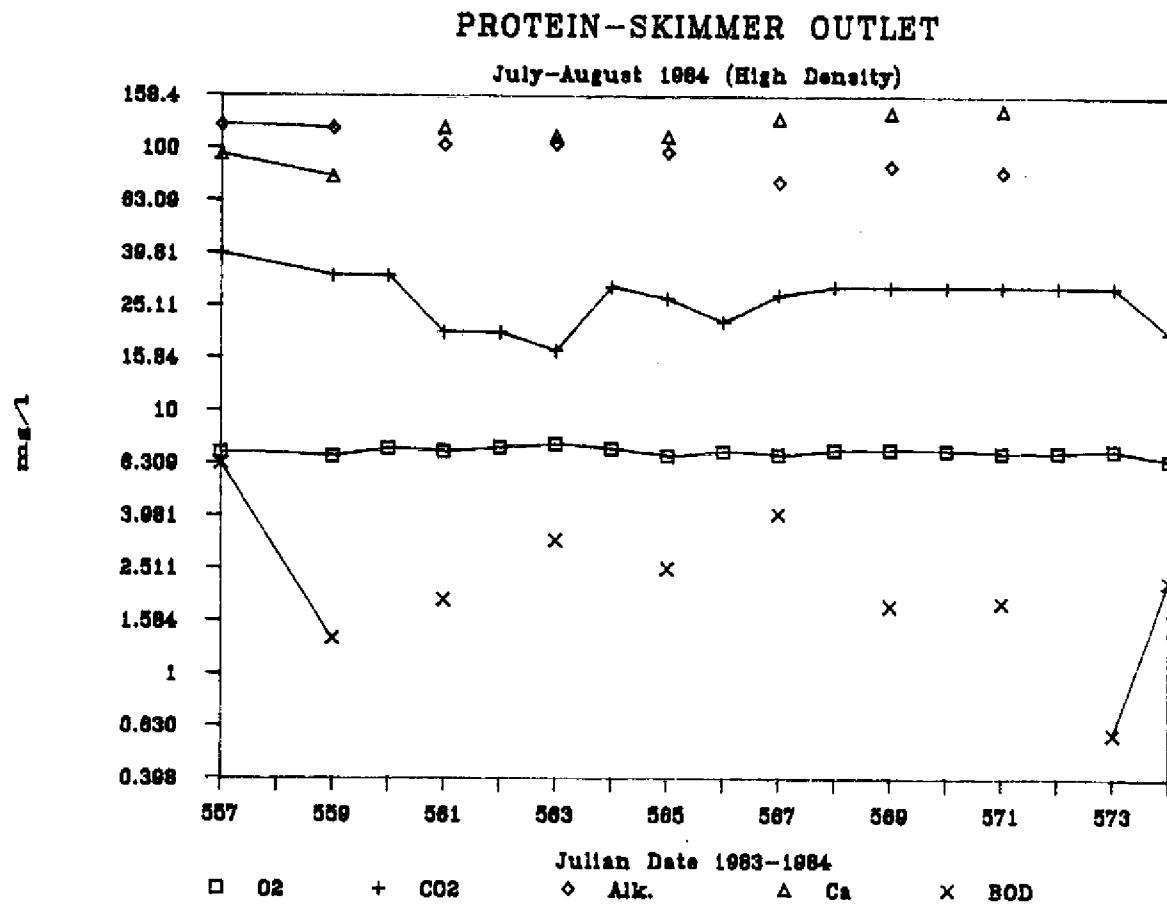
Figure 18. Mean outlet dissolved O<sub>2</sub>, dissolved CO<sub>2</sub>, alkalinity, calcium, and BOD levels for the protein skimmer stocked at high densities (July-August, 1984)
