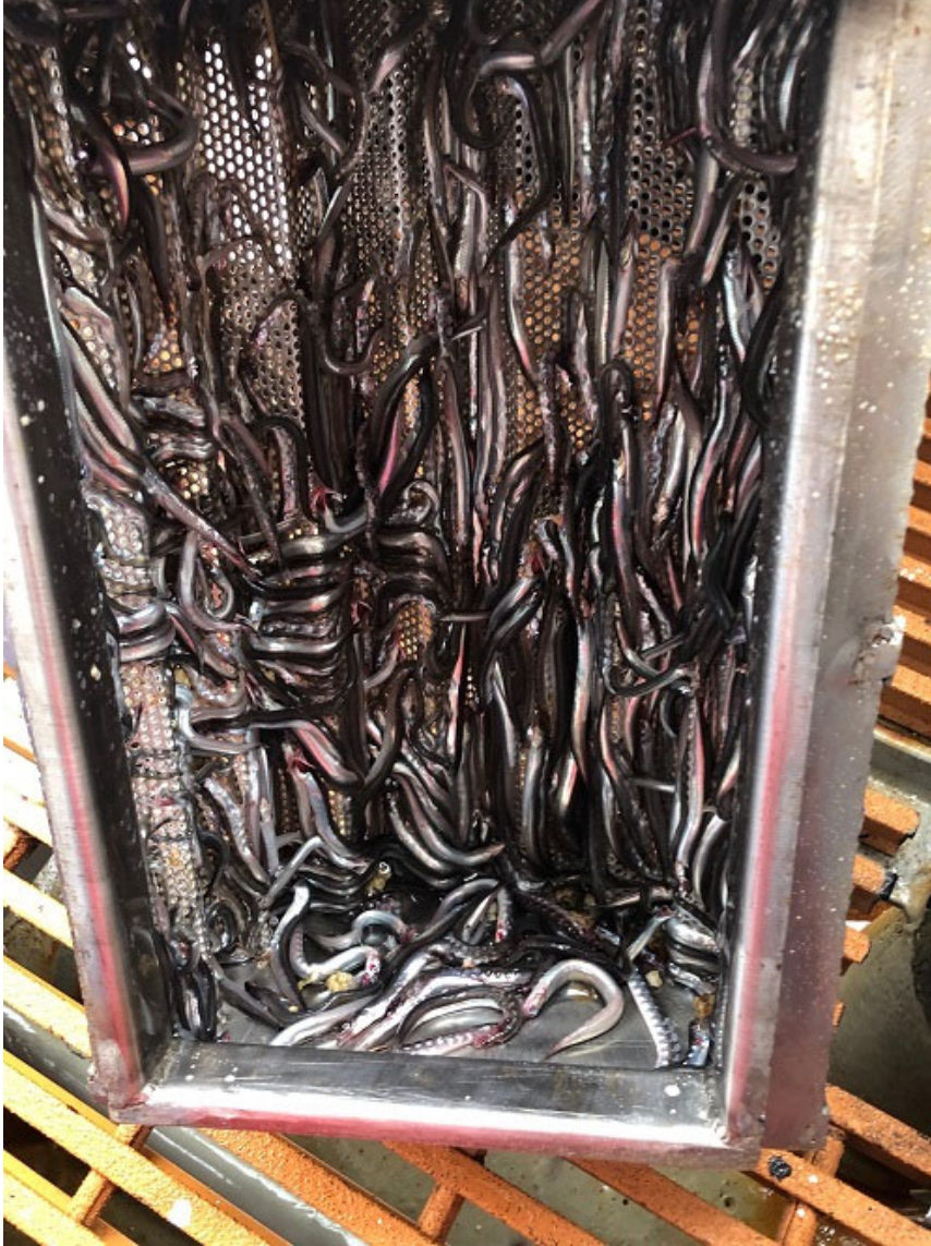
Figure 9. Large numbers of sand lance clogged the strainer of the cooling water intake for the diesel engines of of the Gordon Gunter.
