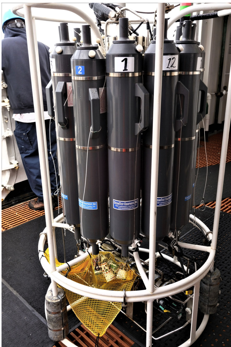
Figure 5. Niskin bottle rosette on the deck of the port side sampling Station aboard the FSV Gordon Gunter.
