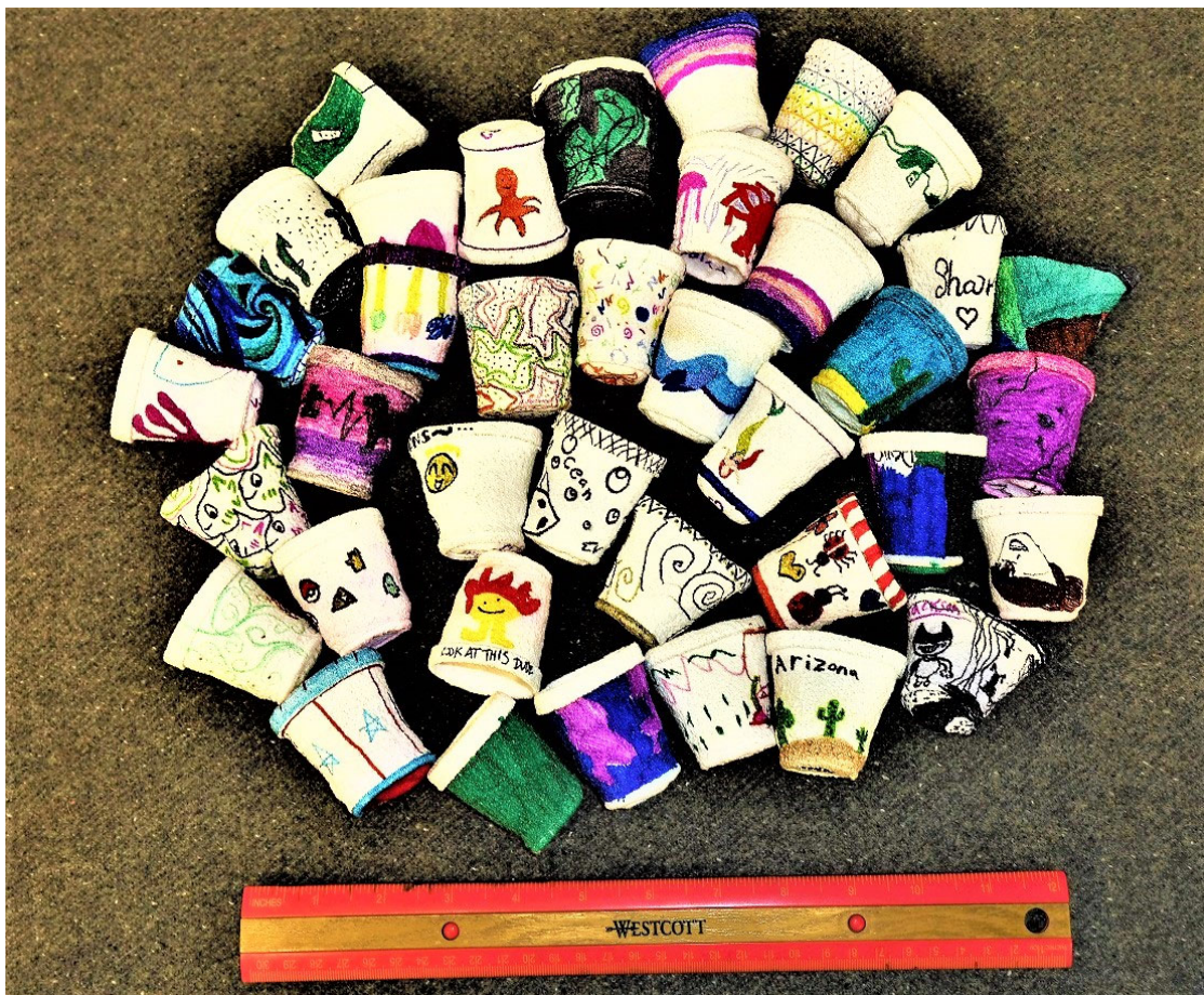
Figure 6. Styrofoam cups decorated by students from the Banner Academy in Tempe, Arizona. After repeated submersions with the Niskin bottle water sampling array they have shrunk to a fraction of their former size, as seen from the 12 inch ruler below them.
