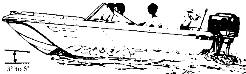
Figure 5A. Weight distribution affects a boat's running angle. For best top speed, all movable weight should be as far aft as possible to allow the bow to come up to a more efficient angle (3° to 5°). However as weight is moved aft, getting on plane becomes more difficult. Moreover, the ride in choppy water may become uncomfortable.
