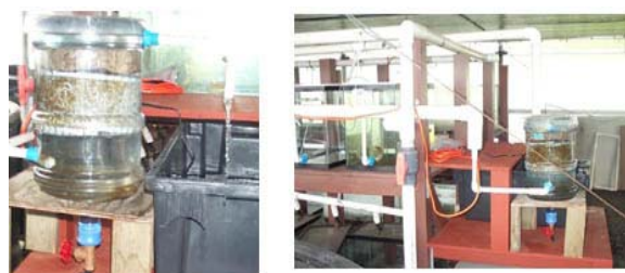
Figure 3. Aquarium shelf biofilter system. Left: close-up of filter vessel showing layers of Bio Fill and crushed coral. Right: system overview. Photo by J. Szyper.
