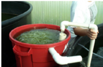
Figure 2. Trash can biofilter. Top: diagram from Backyard Aquaculture in Hawaii. Bottom: working biofilter at UH Hilo farm. Photo by J. Szyper.
