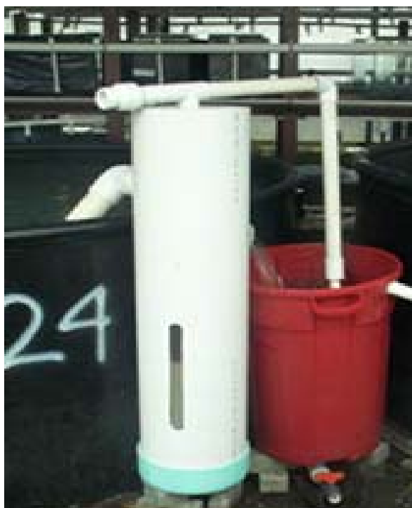
Figure 4. Fluidized bed sand biofilter system including trash can clarifier / pump sump. Photo by J. Szyper.
