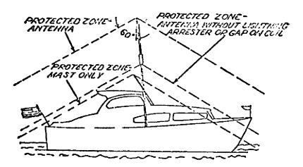
Diagrams above illustrate the "cone of protection" provided by a grounded mast or antenna. This protective zone is largely immine to direct strokes of lightning. No part of the vessel to be protected should extend outside the cone of protection. Thus in the cabin cruiser illustrated, adequate lightning protection is afforded only by the grounded antenna equipped with a lightning arrester or gap on the coil.
