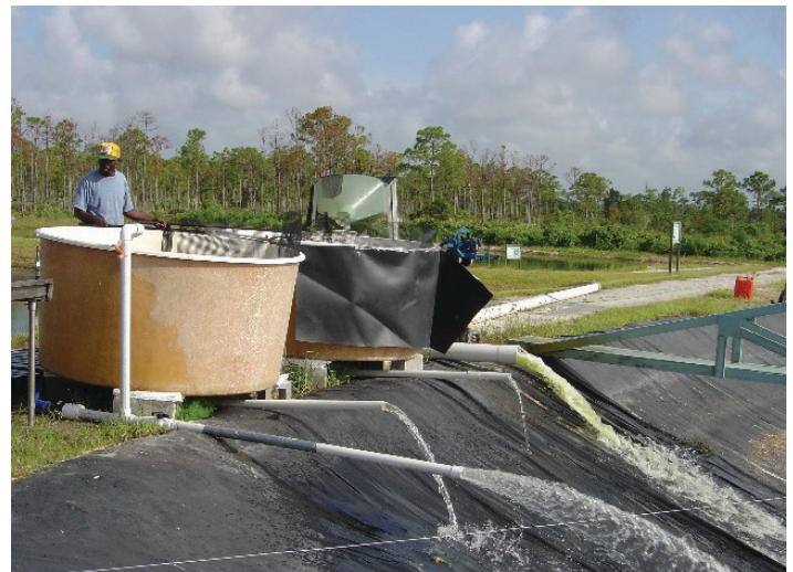
Figure 3. The arrangement of the green dewatering tower and the two round holding tanks on the levee.
