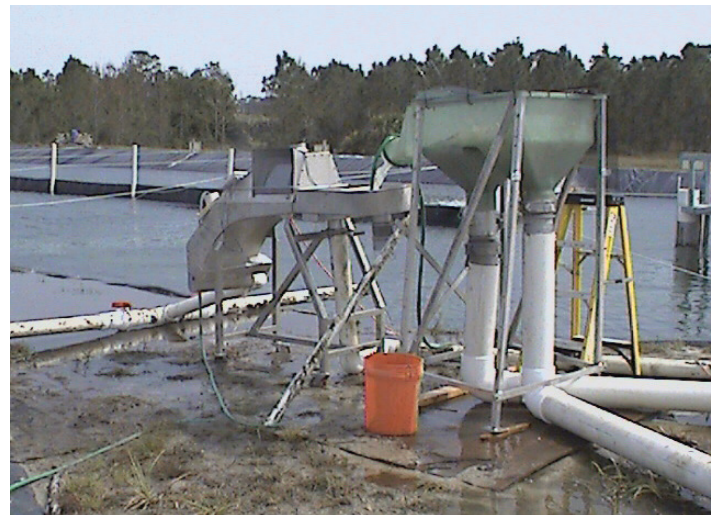
Figure 5. Incorporation of the shrimp counter (left) with the dewatering tower. Credits: Scott W. Grabe
