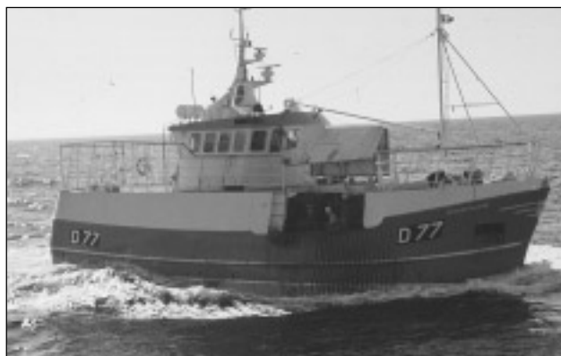
Figure 3. The MFV Peadair Elaine , one of four offshore supercrabber vessels built to fish brown crab off Ireland. The vessel is shooting (deploying) pots.
