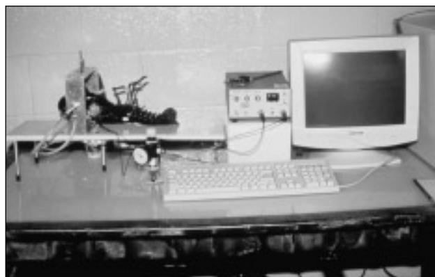
Figure 5. Live lobster in LU Probe test bed. Signal generation and processing unit is at the right side of the figure.
