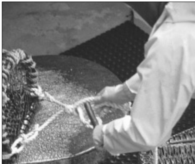
Figure 6. Close-up of the eyesplice and toggle on the crab pot deploy-retrieval system, MFV Peadair Elaine .
