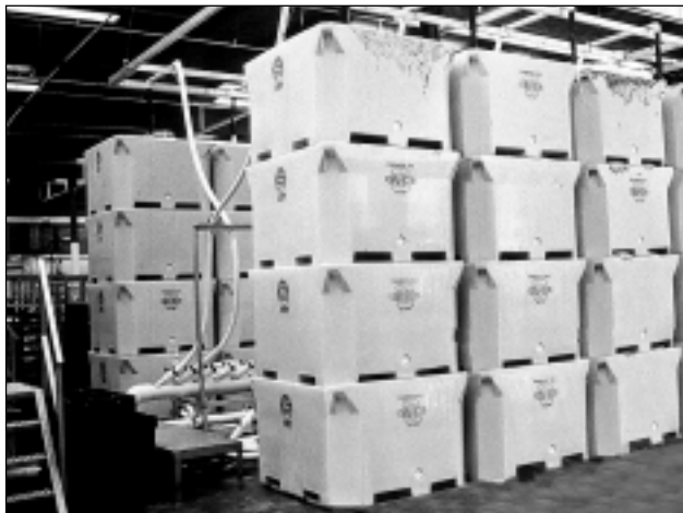
Figure 8. Recirculation system in bulk mussel storage. Stacked tote boxes hold up to 10 metric tons of mussels for re-watering and short-term storage prior to distribution to retailers (David Scarratt photo).
