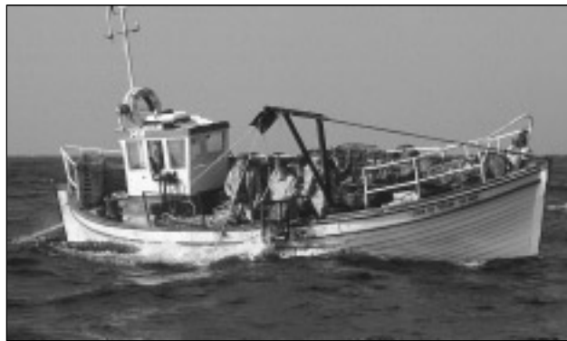
Figure 9. Traditional northwestern inshore crab vessel, of Norse design. This vessel is about 10.5 meters in length with four crew. Landings can be about 150 40-kg boxes per day.
