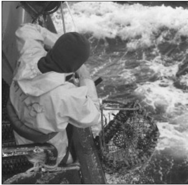
Figure 5. Crewmember at crab pot retrieval station on the MFV Peadair Elaine . The pots are hauled to the surface using a slave hauler, and then pulled aboard.
