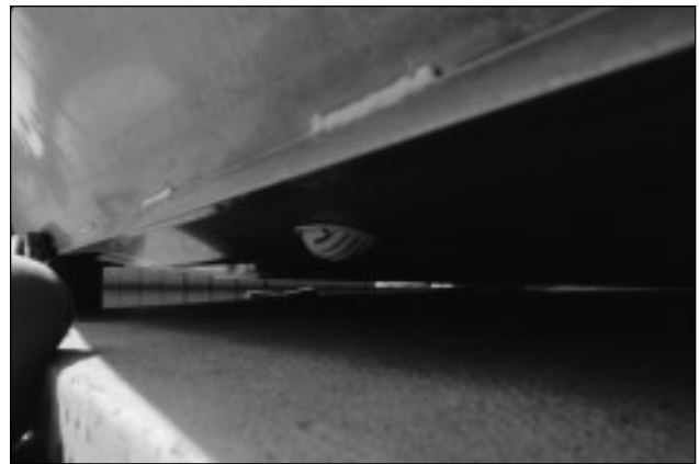
Figure 8. This intake device services the skiff's live tank in a pumpless water system. Water shoots through the forward-facing scoop, through plumbing, and aft to the tank.
