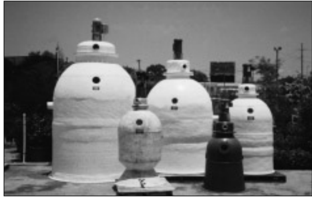
Figure 3. Motorized bead filters.
