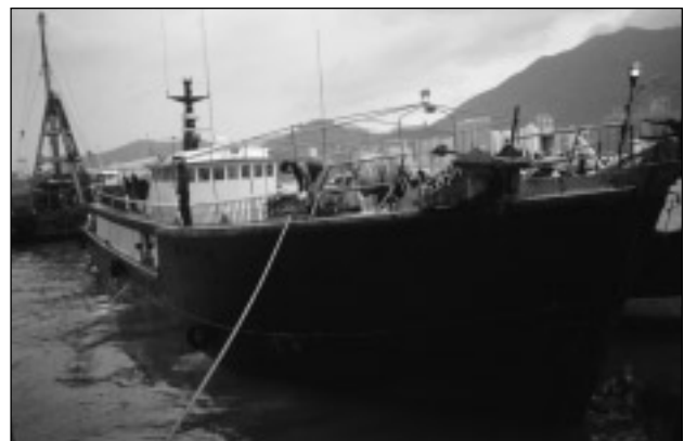
Figure 2. A 120-foot live harvesting vessel is typically equipped with 30-40 live wells and holds about 20 tons of live fish.
