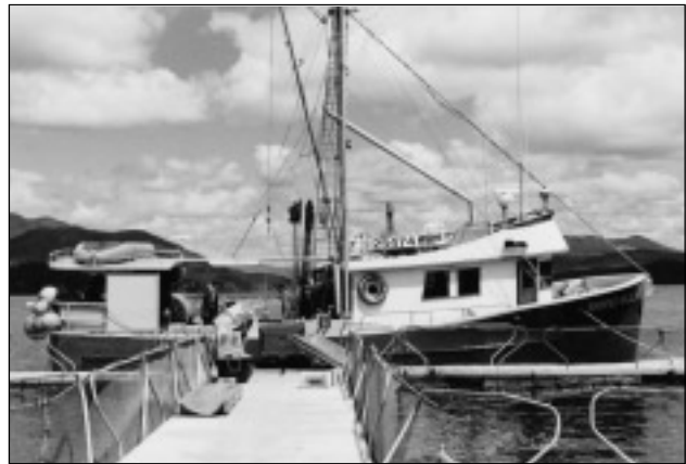
Figure 1. The vessel used in this project is a 50-foot fiberglass longliner, the Triple M II .
