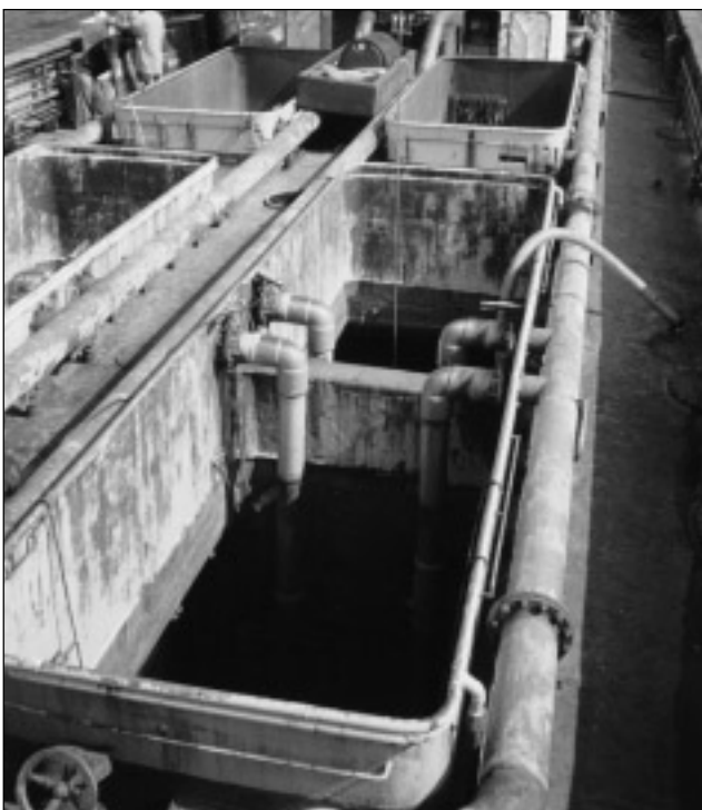
Figure 4. Live well in metal hull fish carrier.
