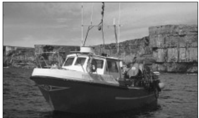
Figure 12. A 15 meter GRP lobster pot vessel fishing off the Aran Islands, west coast of Ireland. The vessel is equipped with twin engines. This type of vessel is becoming increasingly popular for use by the larger, year-round operators, fishing lobster and brown crab.
