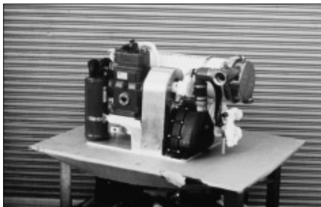
Figure 3. Small integrated refrigeration unit intended for use of small harvesting vessels. Courtesy of Mark Burn, specialist in small-scale refrigeration systems, Integrated Marine Systems, Port Townsend, Washington.
