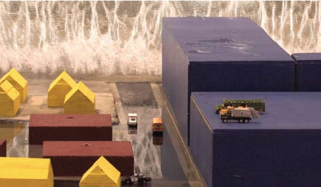
Model of Seaside, OR used by Sea Grant researchers to understand impacts of tsunamis.
