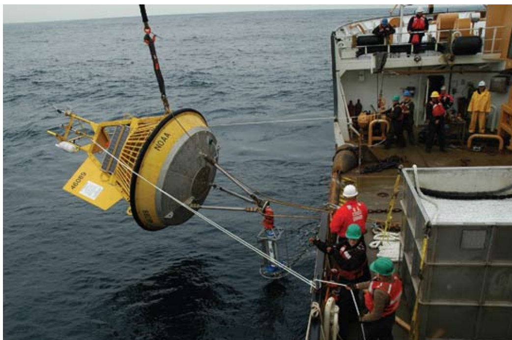
NOAA National Weather Service buoys, like this one, measure ocean and atmosphere conditions and transmit the data via satellite to scientists, who use the data to monitor and predict climatic trends and weather events.
