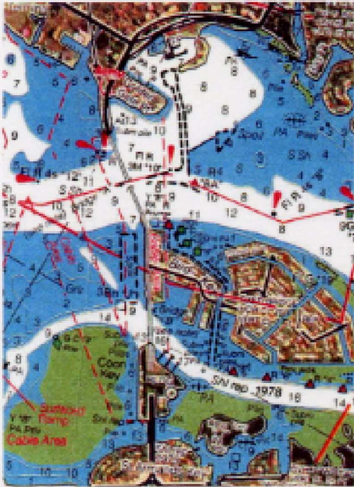
Plate 1. Panels 1, 2 and 3B. Bathymetry shown as spot soundings over white (greater than 6 feet) and blue (less than 6 feet) depth ranges.
