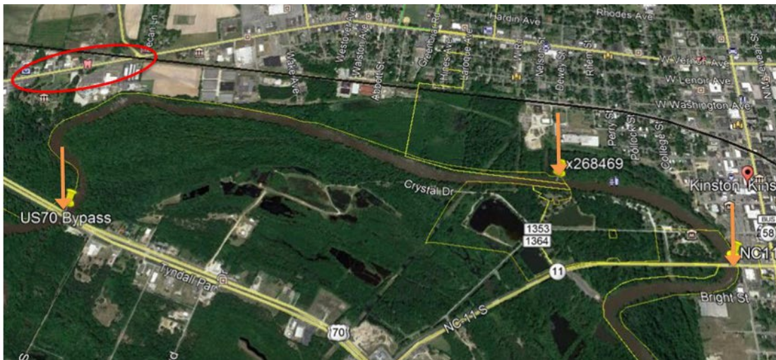
Figure 4-3. HEC-RAS cross sections (indicated by arrows) in the vicinity of W. Vernon Avenue.
