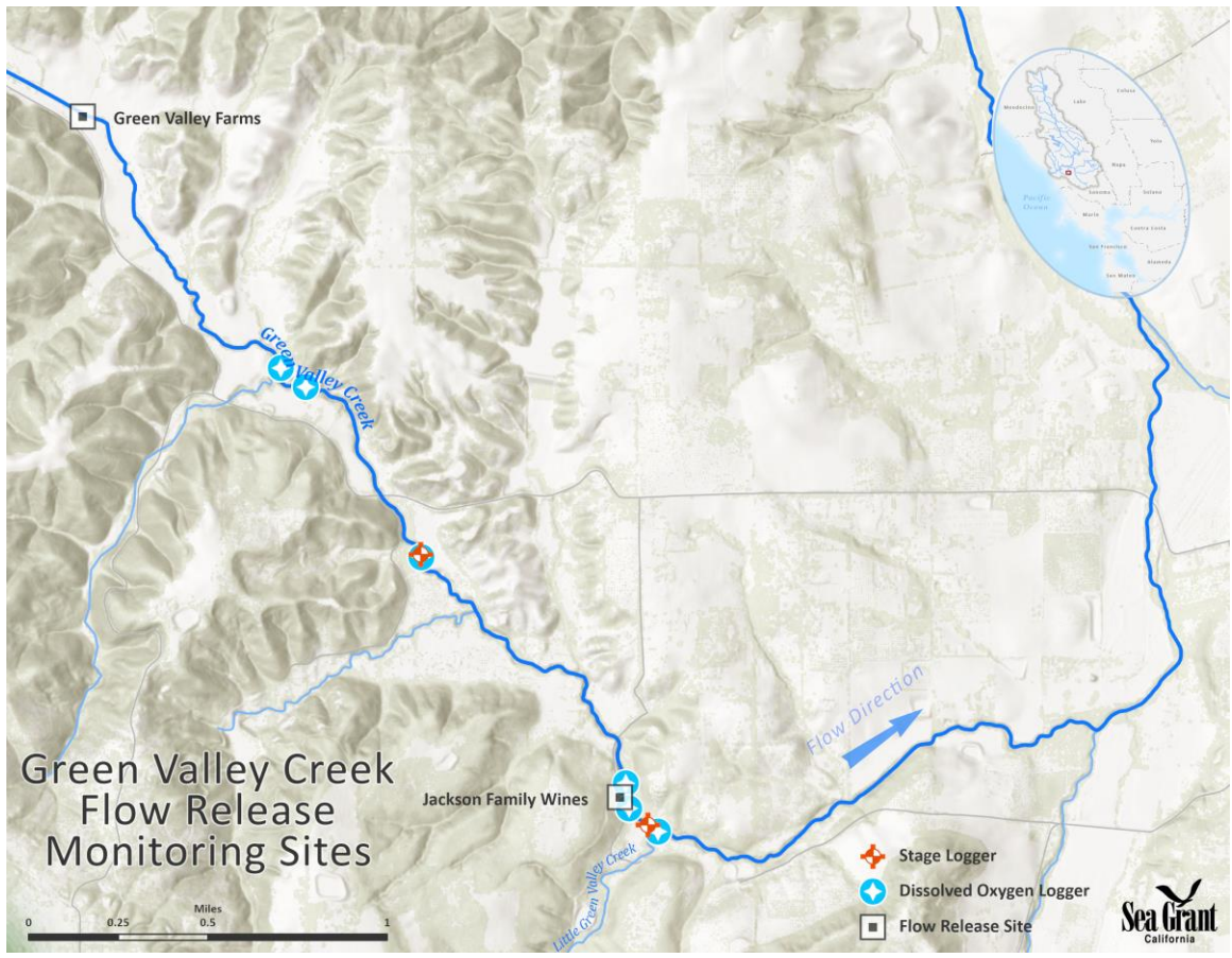
Figure 45. The Jackson Family Wines (JFW) and Green Valley Farms (GVF) flow release sites, and stage (flow) and water quality (DO and temperature) loggers used to monitor release effects in Green Valley Creek, years 2017-2019.
