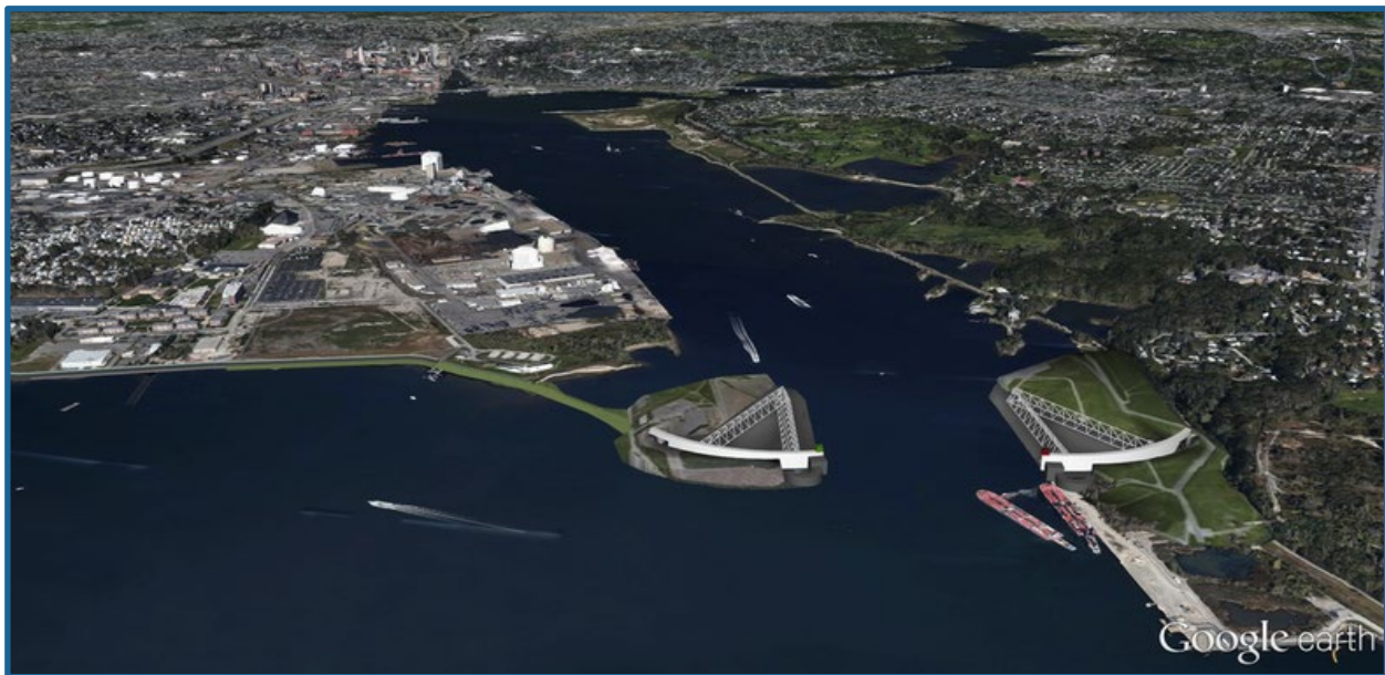
Figure HB-4. Fields Point Barrier Concept to Protect the Entire City from Storm Surge. Simulation based on design used in Rotterdam (Becker et al., 2017).
