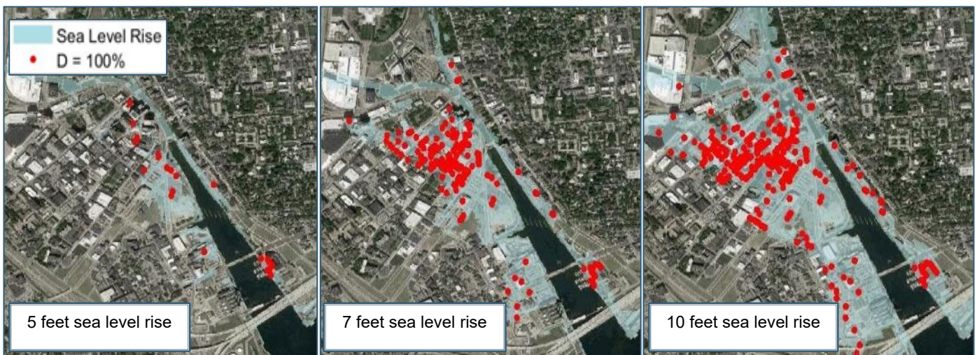
Figure D-2. Projected Damages to Buildings from Sea Level Rise Downtown. The number of buildings behind the barrier that are projected to be damaged 100% increases with sea level rise scenarios: 5 feet rise (26 buildings), 7 feet rise (184 buildings), and 10 feet rise (363 buildings) (URI, 2018a).
