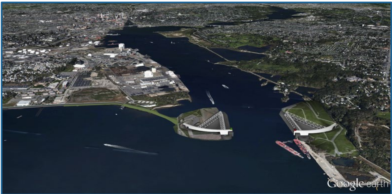
Figure P-4. Fields Point Barrier Concept. Simulation based on design used in Rotterdam (Becker et al., 2017).
