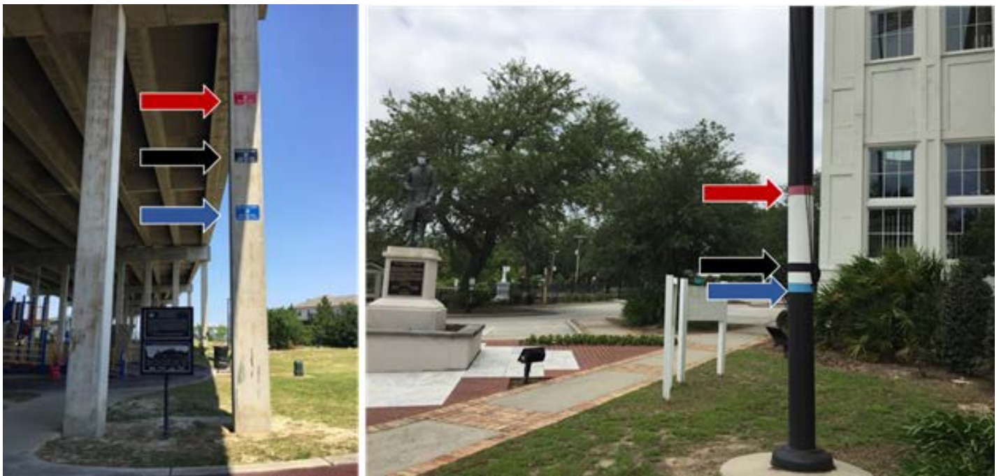
FIGURE 1: High Water Marks at two locations showing the colored lines. Corresponding colored arrows point to the colored high water mark lines. Red indicates Hurricane Katrina, blue indicates Hurricane Camille, and black indicates the base flood elevation (BFE).
