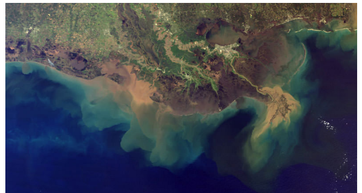
FIGURE 3. Scientists use satellite imagery to look for oil spills and algal blooms. Discharge from rivers, like the Mississippi in the middle of the image, can change the color of water making it difficult for scientists to see their target. (NASA)
