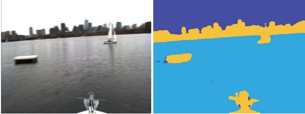
Figure 8: Left Image: Camera image of floating obstacle and sail boat Right Image: Machine learning scene segmented output. Pixel representation, Purple = Sky, Yellow = Obstacle, and Blue = Open Space
