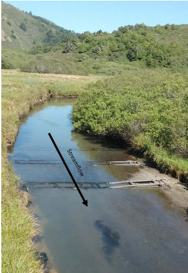
Figure 2. Paired flat-plate antenna array on Willow Creek.
