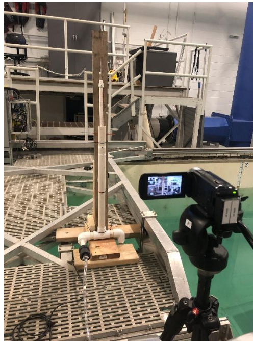
Figure 4: Alpha Model Kinovea Setup
