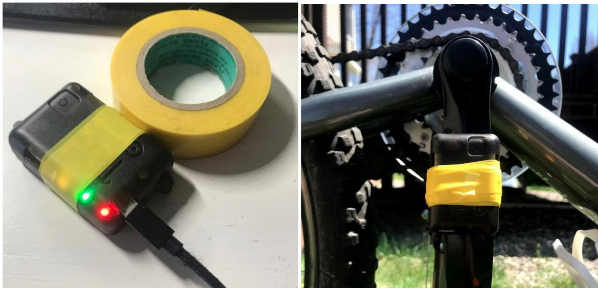
Figure 33: a) NGIMU when connected to the computer b) NGIMU fixed to the crank arm of the bike.
