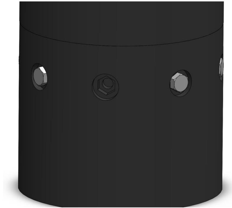
Figure 20: 5/16 Bolt Mounting Hole
