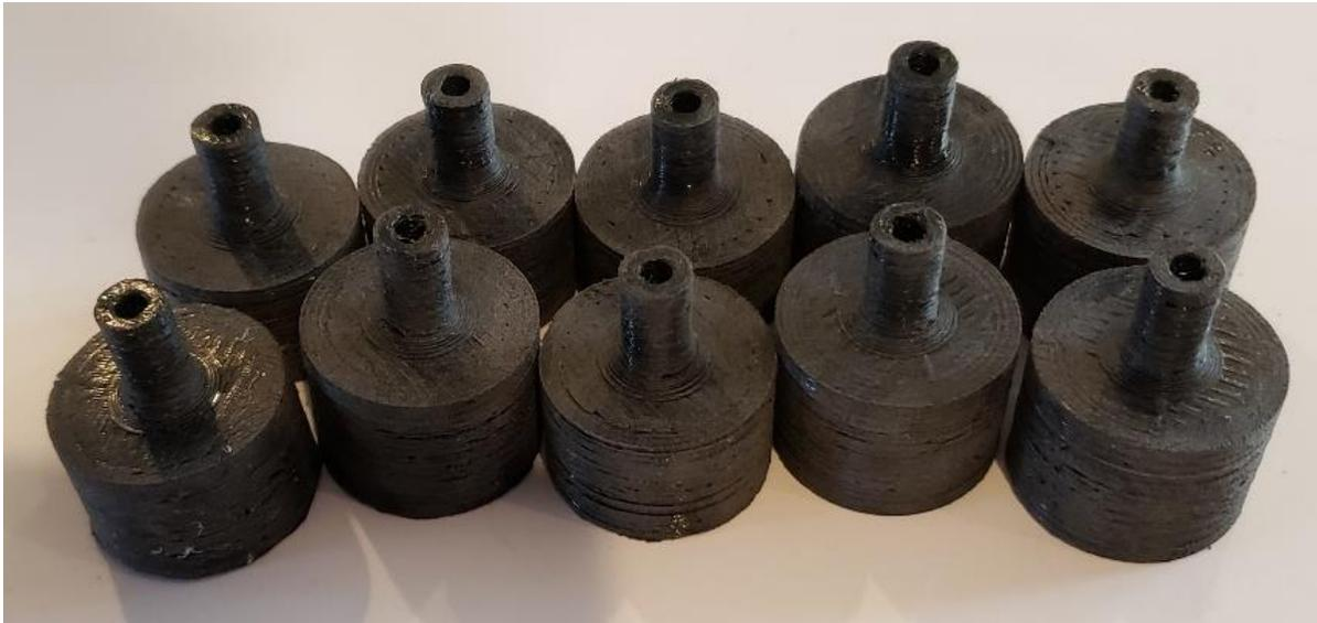
Figure A-5: 3D Printed Pressure Vessels- Final Product
