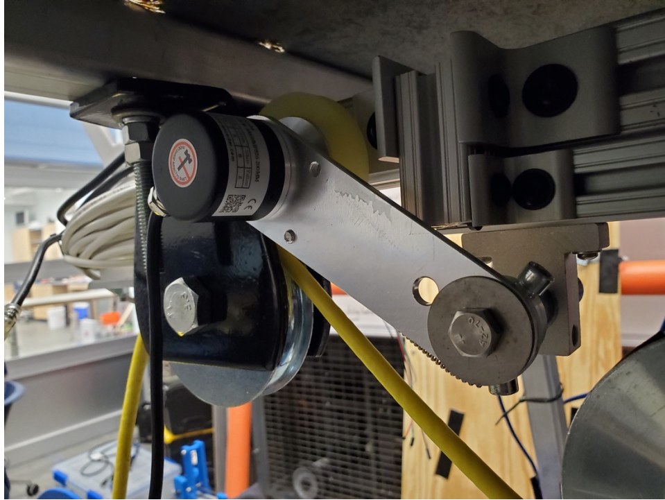
Figure 10: The rotary encoder mounted to run with the tether. Contact with the tether is maintained with a tension spring to ensure the wheel is always moving without slip
