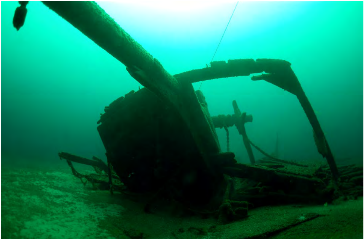
Figure 22. Cross-planked bow of Ocean Wave (Wisconsin Historical Society).
