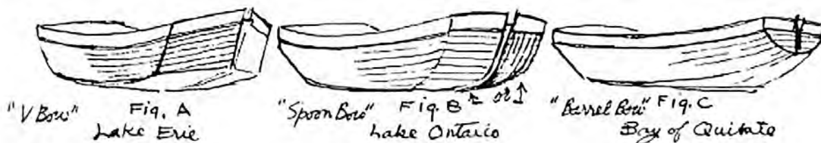
Figure 1. Various scow bow structures (Loudon Wilson).
