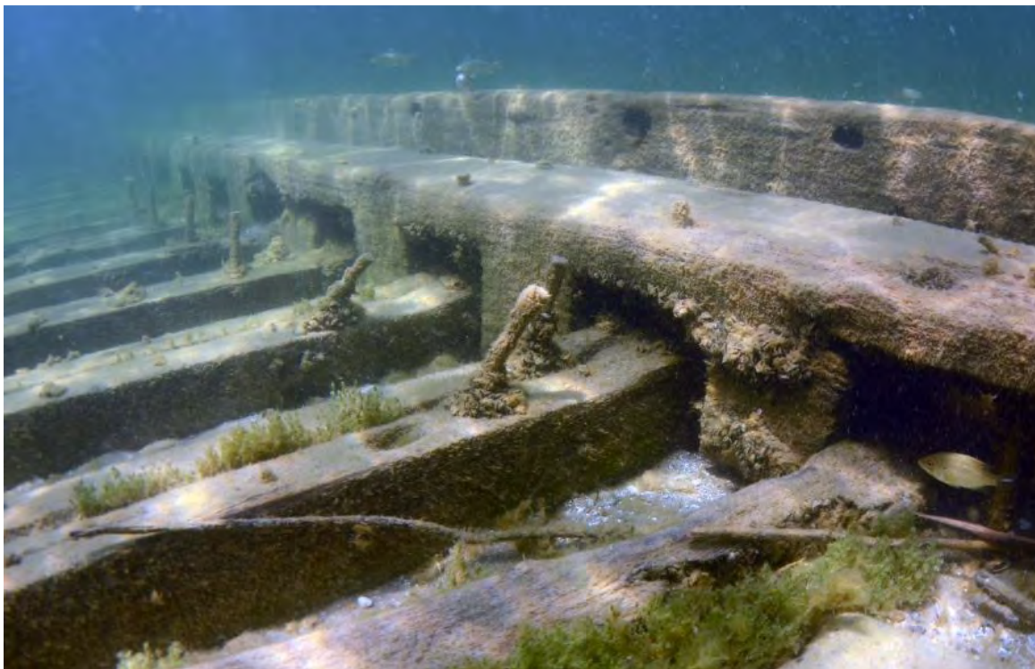
Figure 4. Pocket pieces on the port centerboard trunk of the General Winfield Scott's lower hull. (Wisconsin Historical Society)
