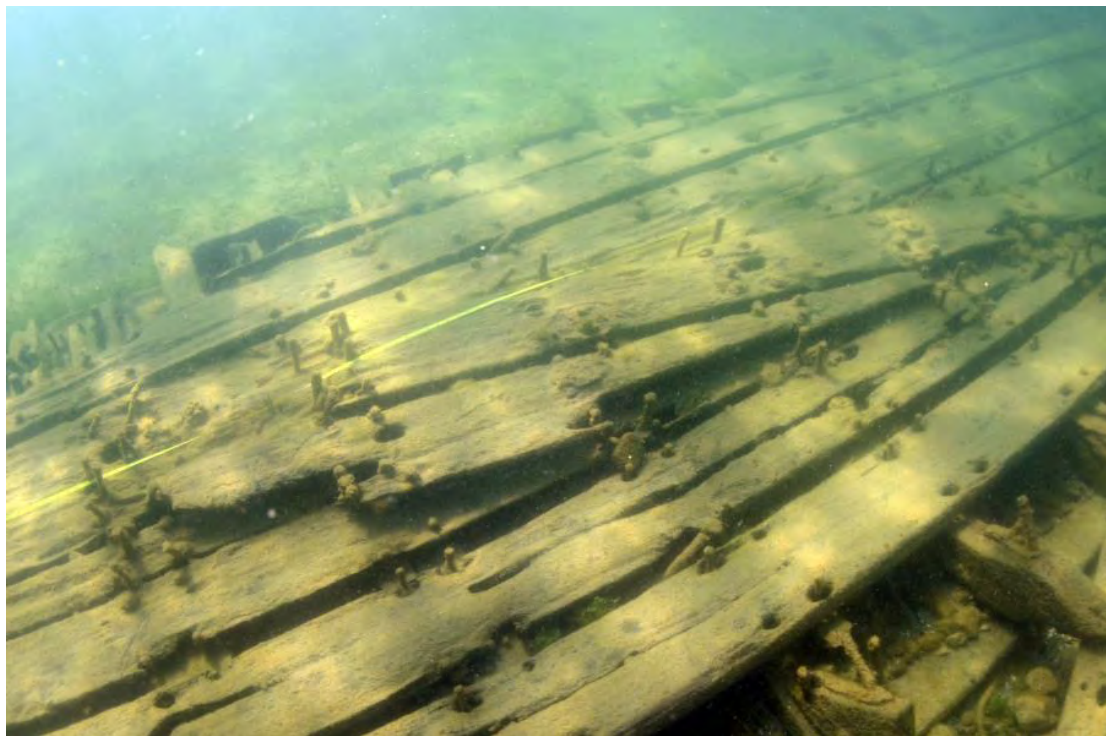
Figure 9. Hogging arch located on the starboard hull. (Wisconsin Historical Society)
