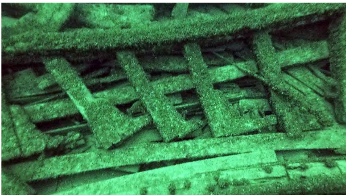
Figure 39. Transfer's stanchions with support knees (Tori Galloway)
