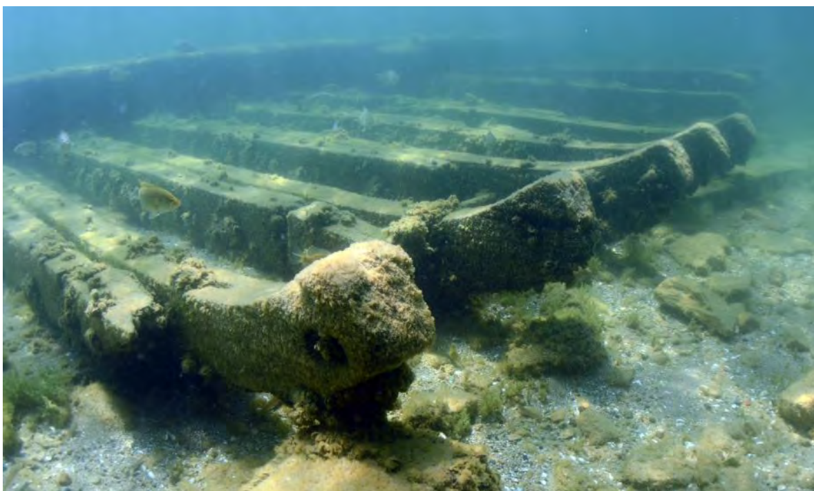
Figure 2. Lower hull of General Winfield Scott - keelson, floors, and turn of the bilge (Wisconsin Historical Society)
