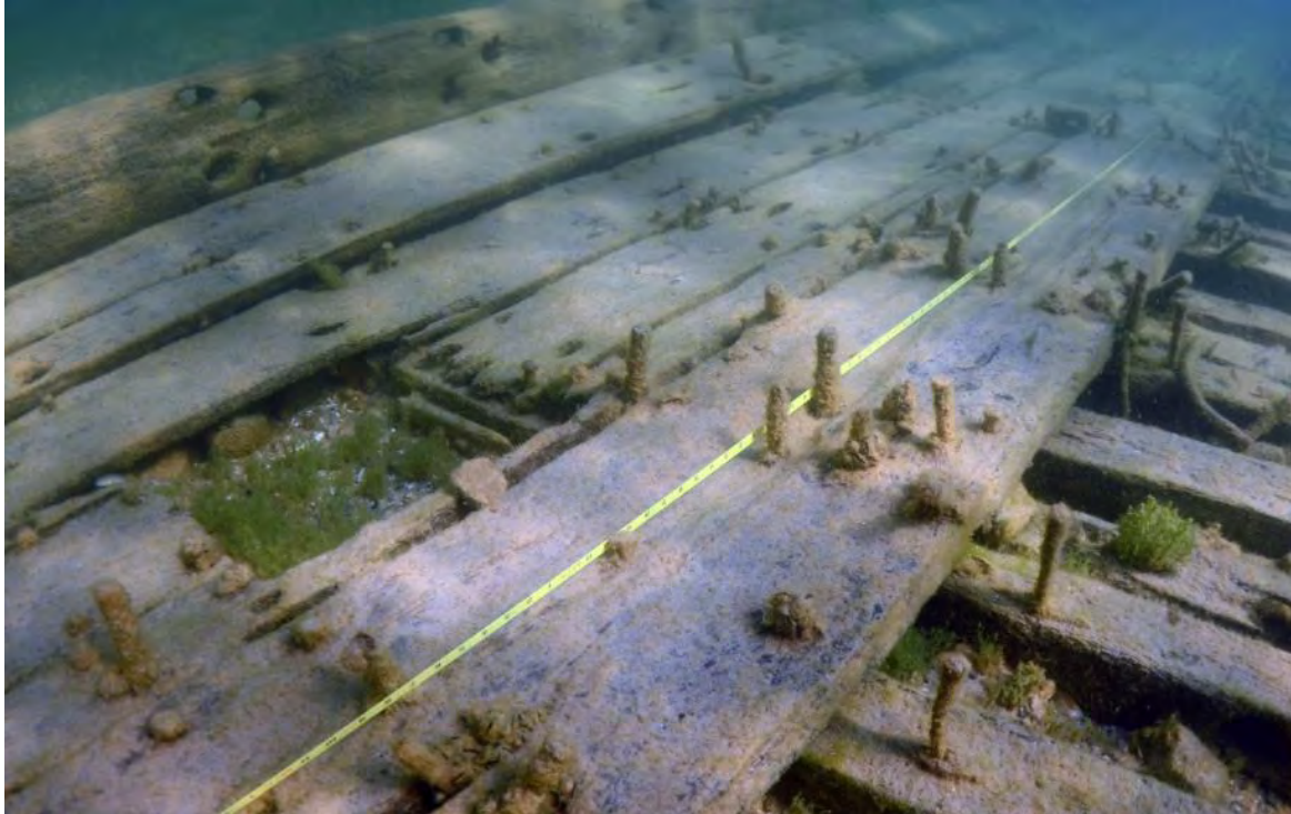
Figure 6. Starboard hull section of the General Winfield Scott showing a bilge stringer, ceiling planking, lumber port, and frames. (Wisconsin Historical Society)
