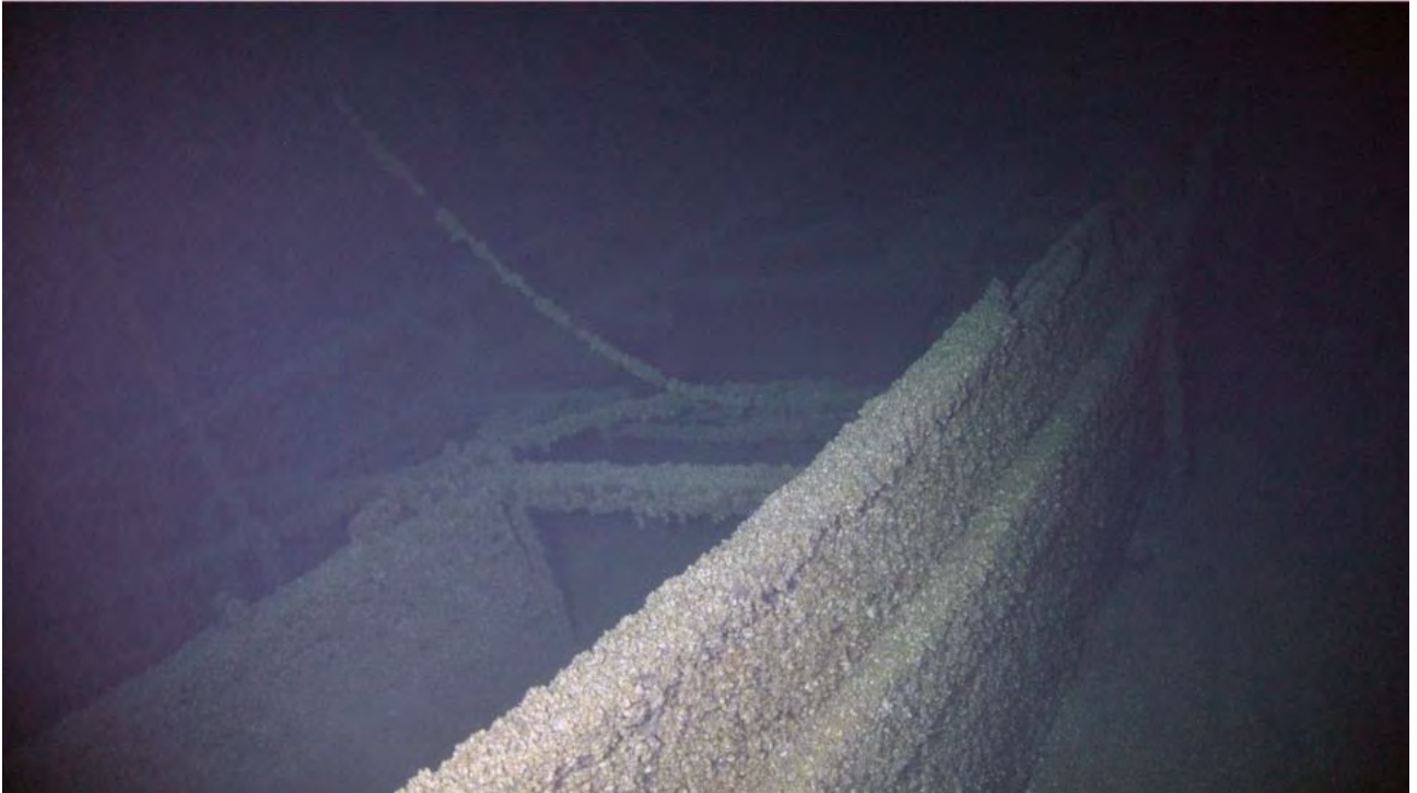
Figure 54. Port side of the vessel looking aft, showing deck beams, centerboard trunk, bulwarks and rubrail (Marine Imaging Technologies)
