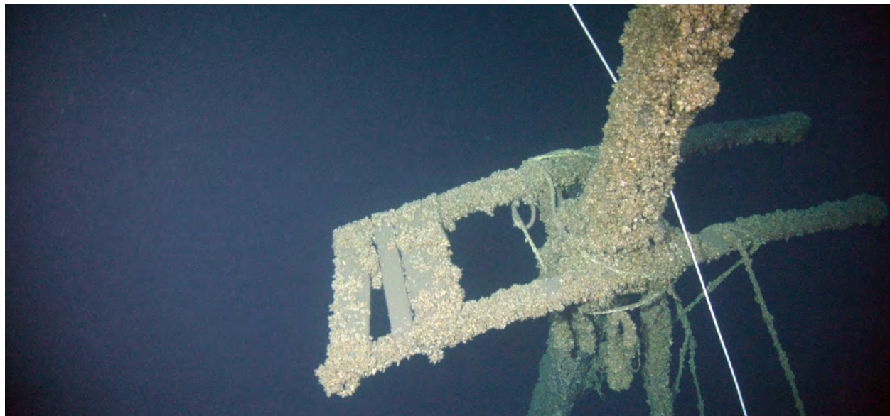
Figure 59. Tennie & Laura's foremast trestletree (Marine Imaging Technologies)
