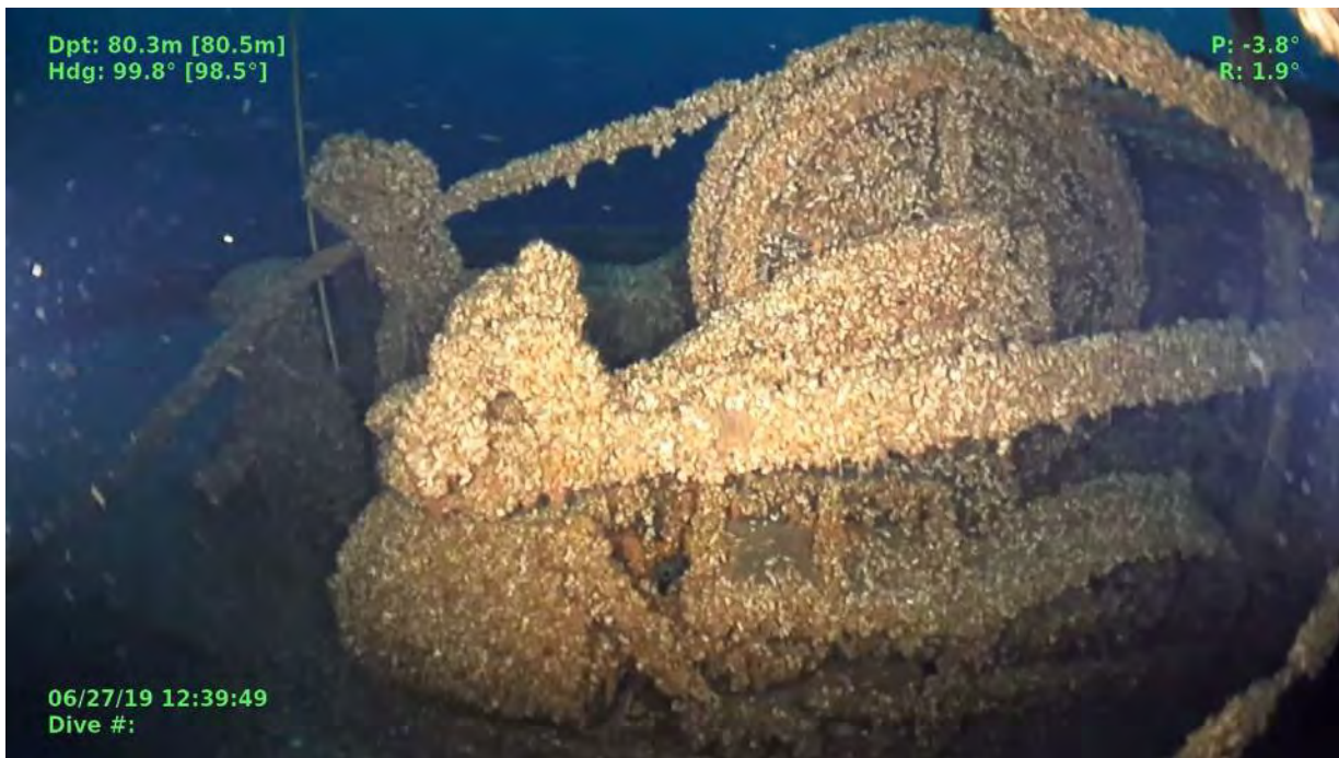
Figure 28: Steam winch located on the aft deck (Crossmon Consulting LLC)
