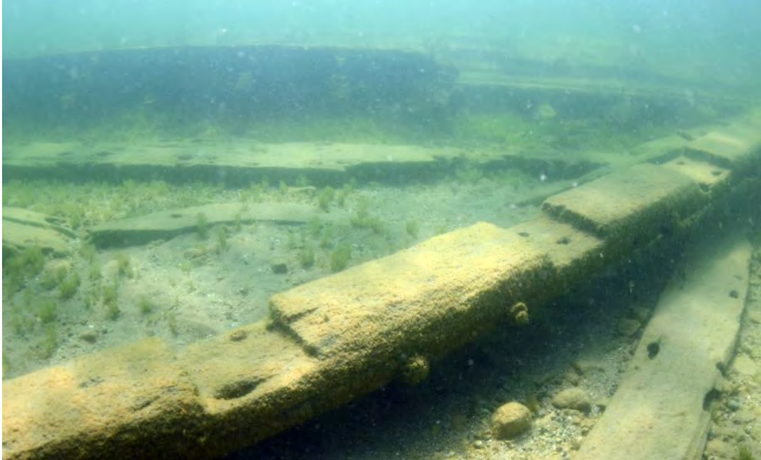
Figure 8. Bilge stringers located at the turn of the bilge (Wisconsin Historical Society)
