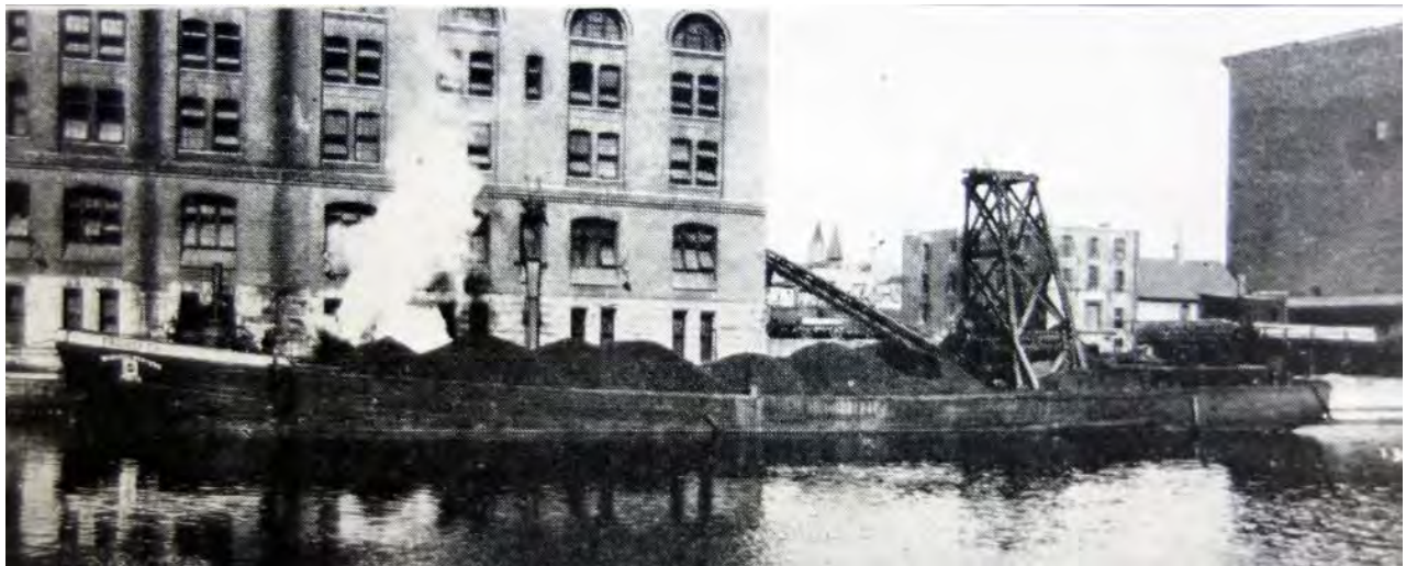
Figure 34. Transfer equipped with self-unloading machinery transfers coal to the Commonwealth powerhouse (Rail and Wire 1916)
