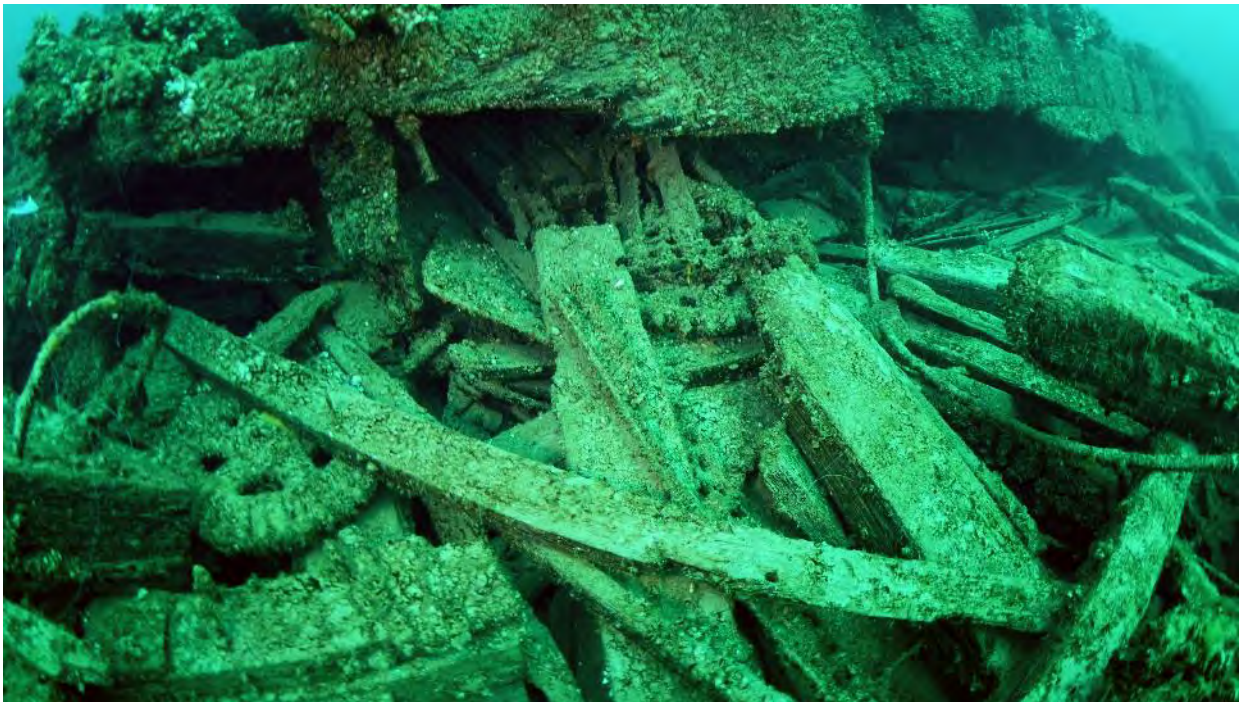
Figure 44. Transfer 's bevel gears and athwartship conveyor, with sprocket gear and roller chain (Wisconsin Historical Society)
