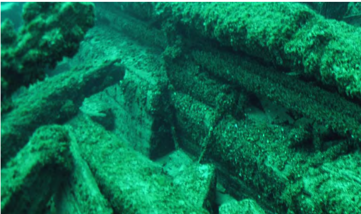
Figure 38. Transfer 's keelson structure and triangular support (Wisconsin Historical Society)
