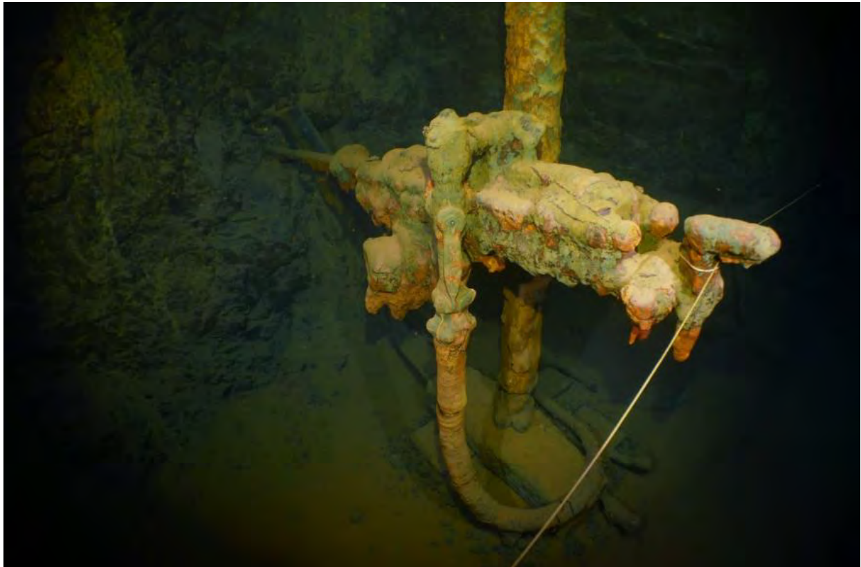
Figure 85. Post drill with bit remaining in the wall of the stope (Leah Potts)
