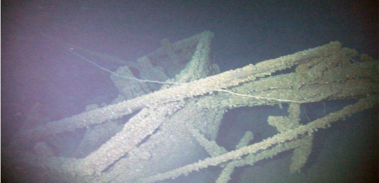
Figure 55. Tennie & Laura's V-shaped bow, windlass, jibboom, and anchor (Marine Imaging Technologies)
