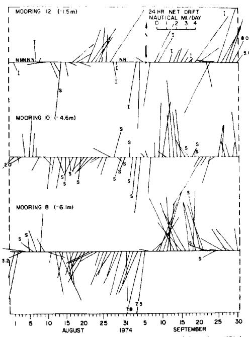
Figure 7: Sequential 24-hour net-drift vectors for August and September, 1974 from moorings 12 and 10 located 2 km offshore and mooring 8, 7.5 km offshore; N = no data, I = data incomplete and S = speed data incomplete, assume 0.1 kts.
