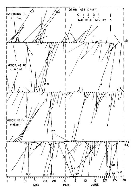
Figure 5: Sequential 24-hour net-drift vectors for May and June, 1974 from moorings 12 and 10 located 2 km offshore and mooring 8, 7.5 km offshore; I = data incomplete and S = speed data incomplete, assume 0.1 kts.
