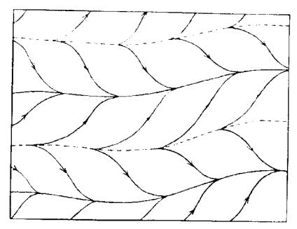
Figure 3. Surface view of streamlines of convection cells with lines of upwelling (divergence) shown as broken lines, and of downwelling (convergence) as full lines.
