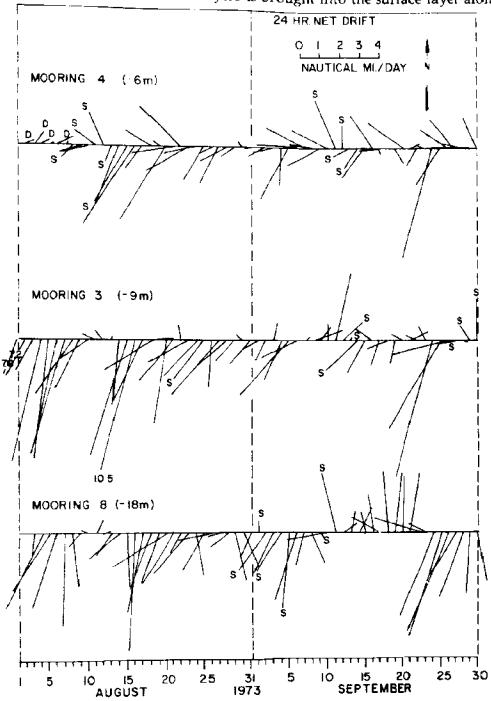
Figure 10: Sequential 24-hour net-drift vectors for August and September, 1973 from moorings 4 and 3 located 2 km offshore and mooring 8, 7.5 km offshore; D = direction data incomplete and S = speed data incomplete, assume 0.1 kts.
