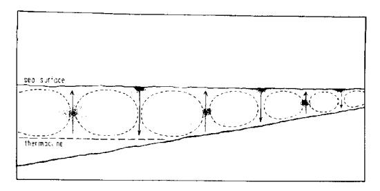
Figure 2. Diagram of convection cells over thermocline and shoaling bottom. Regions where organisms accumulate are dotted. P = non-motile organisms with positive sinking velocity; Q = motile or buoyant organisms.
