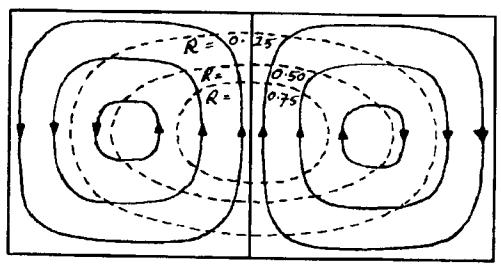
Figure 1. Diagram of streamlines in convection cells with boundaries of regions of retention for three values of R. (from Stommel 1949).
