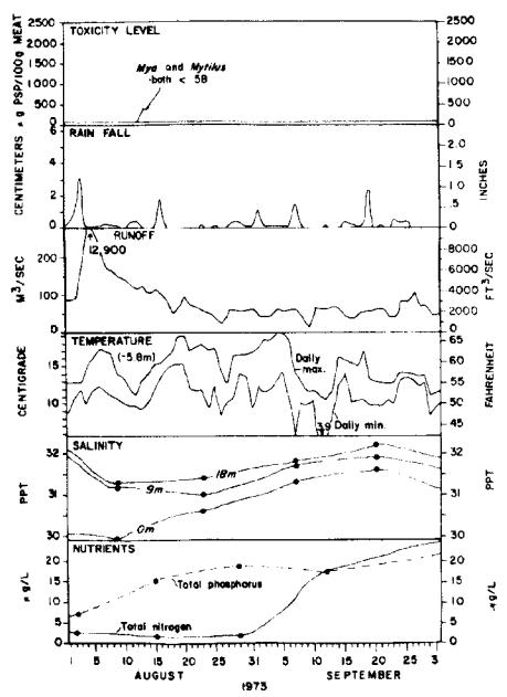
Figure 9: Toxicity levels of shellfish in Hampton Harbor, local rainfall, runoff from the Merrimack River, temperature at mooring 4, high water salinities 2 km offshore, and nutrients 1 km offshore for August and September, 1973.
