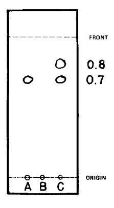
Fig. 3. TLC analysis of crude G. breve toxin, fraction  $I_C$  and tygon tubing extract. TLC plate: silica gel 60 F-254 (E. Merck). Solvent system: toluene:ether:ethyl acetate: acetic acid (80:10:10:0.2). A: crude toxin (extracted in an all-glass system from red-tide sample), B: purified toxic fraction  $I_C$ , C: tygon tubing extract.
