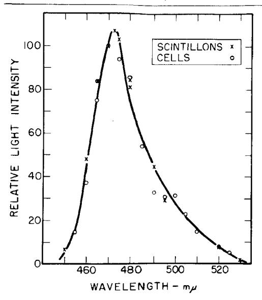
Figure 2: This figure illustrates the similarity between the cotor of light emitted by isolated scintillons and by living Gonyaulax cells. The spectra were obtained using a small Bausch and Lomb monochromator with a second photomultiplier at the entrance slit to monitor the intensity of the incident light. No corrections for phototube sensitivity and monochromator efficiency have been made.
