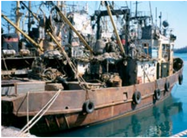
The 70 foot small fishing seiner (MRS) was the workhorse of the Soviet inshore fleet and continues to contribute to catches of bot-tomfish and crab (T. Johnson).
