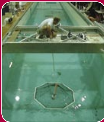
A UNH scientist tests a model cage in a flume tank. Engineers at Ocean Spar Technologies worked with researchers at UNH to test the SeaStation fish cages.
