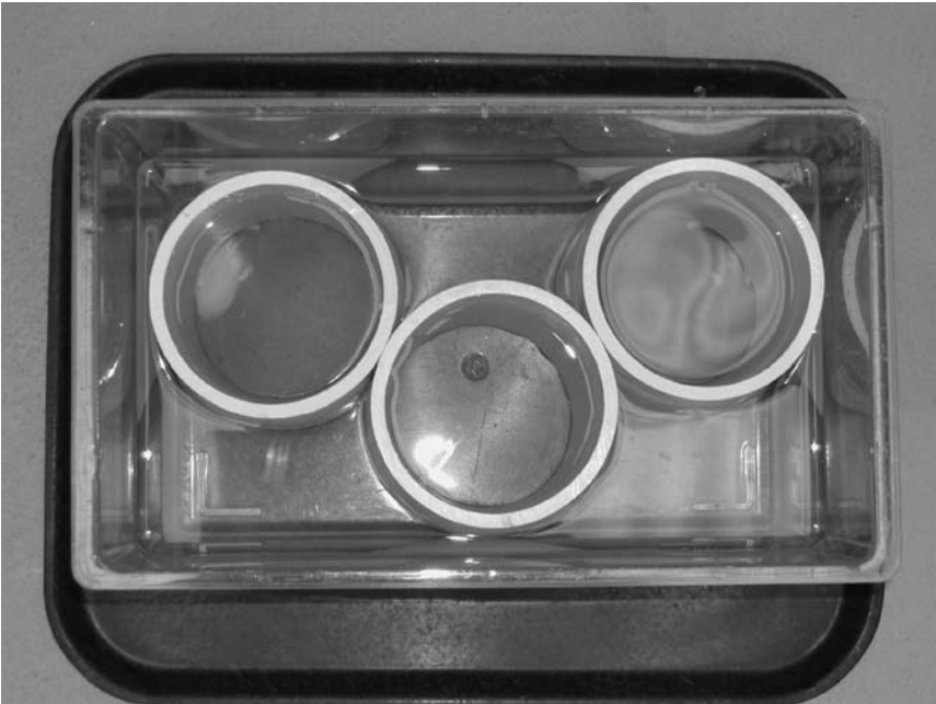
Figure 1. Red king crab larval culture system. Each treatment consisted of a 10 L plastic aquarium filled with 9 L of filtered seawater, containing three PVC cylinders 100 mm in diameter and 150 mm long with a disc of 670 \mu\text{m} nylon mesh attached to the bottom with silicon adhesive.
