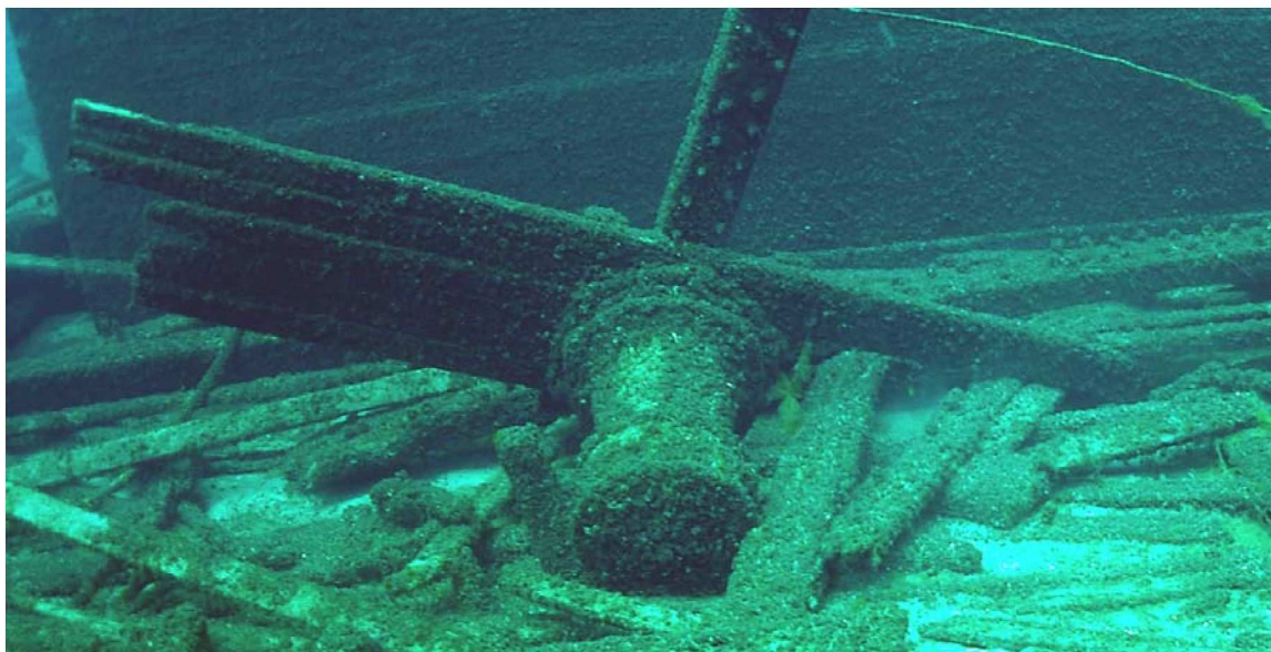
Figure 12. Inverted capstan mounted atop capstan partners and deck beam. Photo by Tamara Thomsen.
